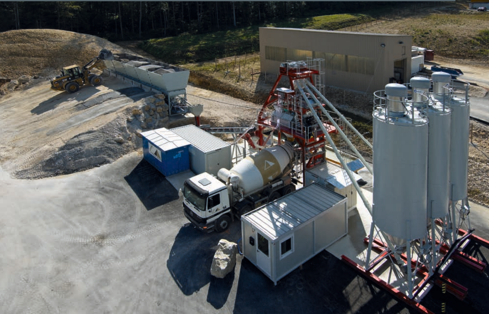
Top Fig: Universal NG 300 with the Amix3_5.00A asphalt mixer Maximum mixer capacity: 5 t/h Bottom Fig: The JustWhite concrete mixing system with the Amix2_3.00SB with a capacity of 1.5 m 3 / batch
