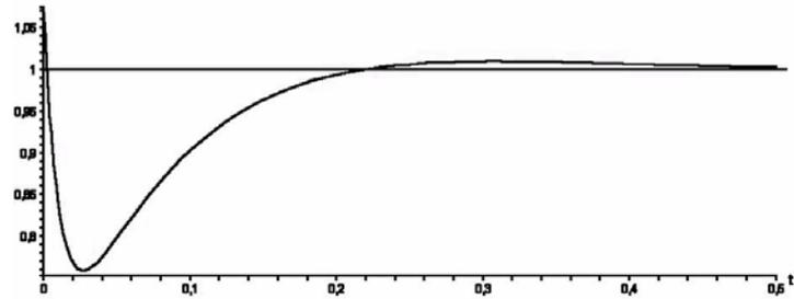
Fig. 8-3 controller operation with D-term too high
