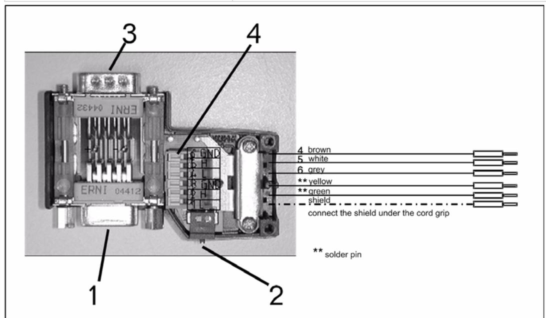
Fig. 9-17 pin assignment LSB plug
