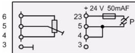
\* At steam pressure: actual value to terminal 3, 4 and 5 and terminal 20 and 21 short circuited. To switch off the internal firing-rate controller, terminal 19 and 21 short circuited.
