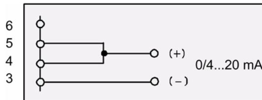
Fig. 9-10 Connection external firing-rate controller
