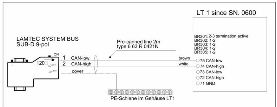
Fig. 9-14 LSB connection ETAMATIC to LT1 from SN 600 on
