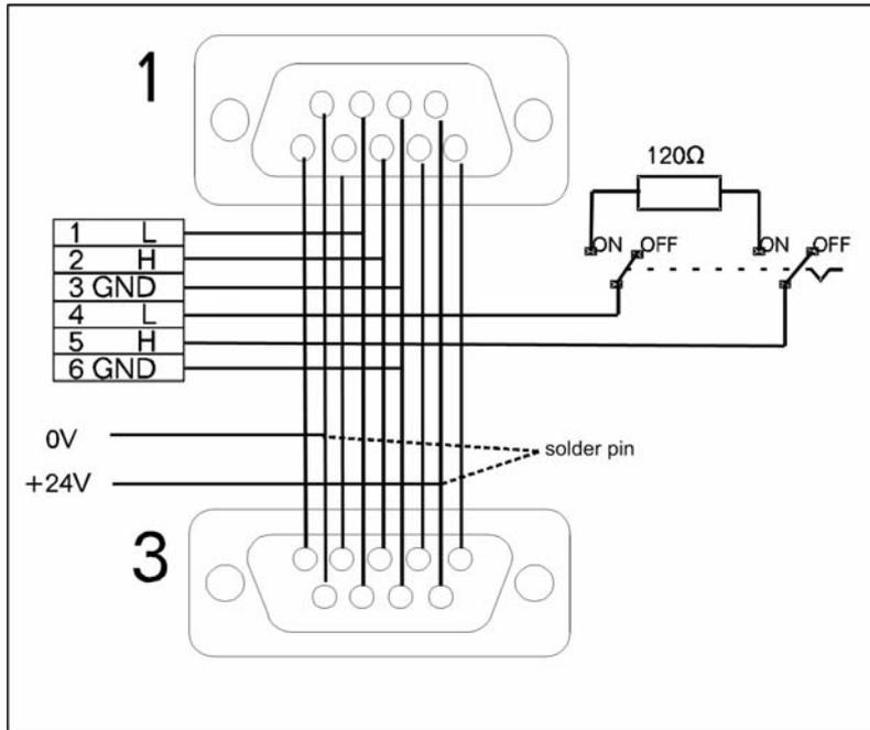
Fig. 9-18 pin assignment LSB plug
