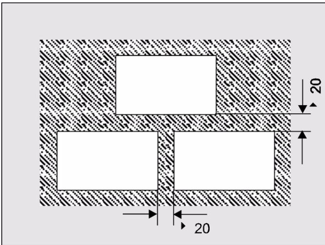
Fig. 9-29 Minimum distances in the case of several cut-outs
