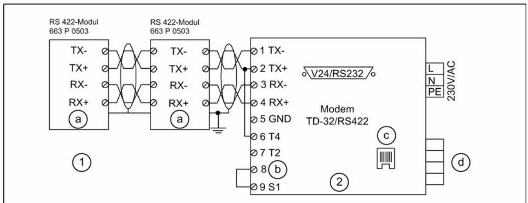
Fig. 9-20 connection diagram modem for remote control
