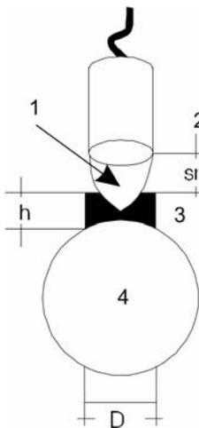
Fig. 9-24 typical arrangement of attenuating element, sensor and shaft.
