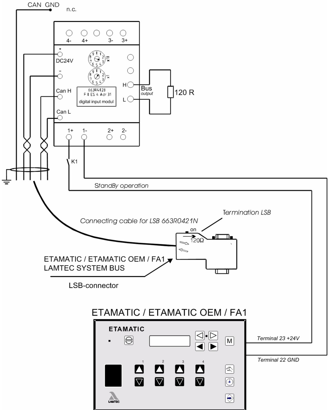
Fig. 8-7 Switching in Standby mode via LSB module
