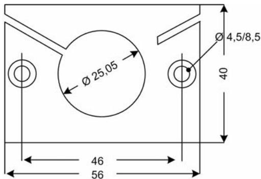
Fig. 9-35 Mounting clip for FFS 06... see also the documentation of the flame scanner FFS05 (DLT7501 and DLT7503)
