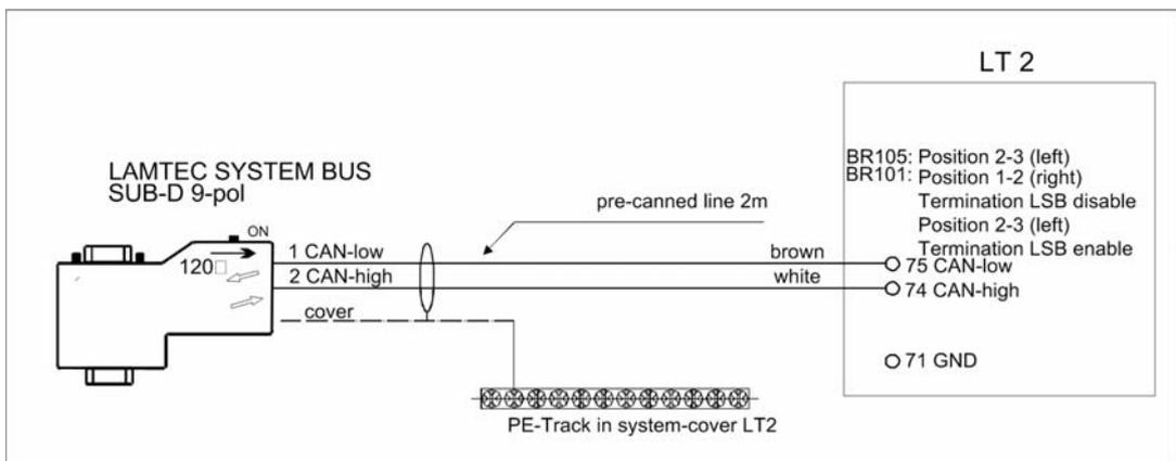
Fig. 9-12 LSB connection ETAMATIC to LT2
