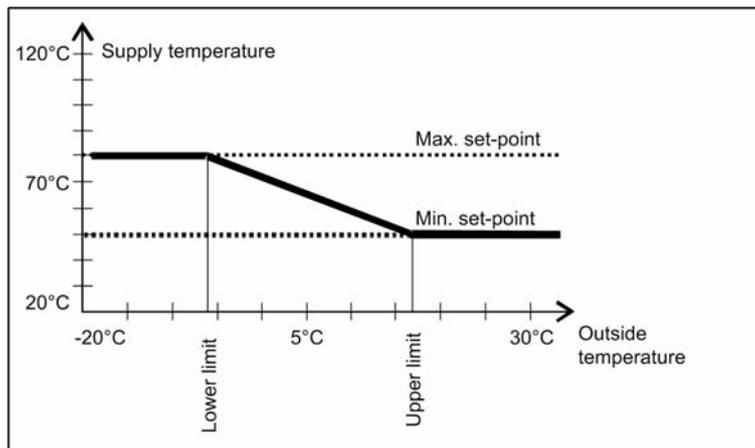
Fig. 7-1 Control by atmospheric conditions
