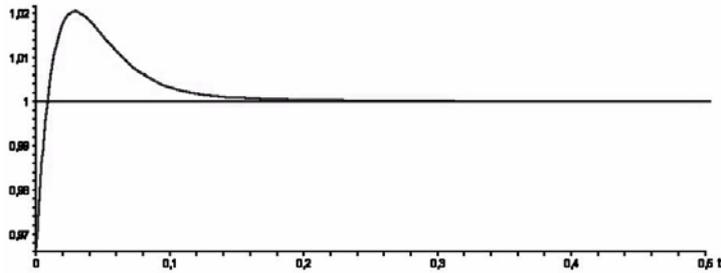
Fig. 8-1 controller operation with P-term too high
