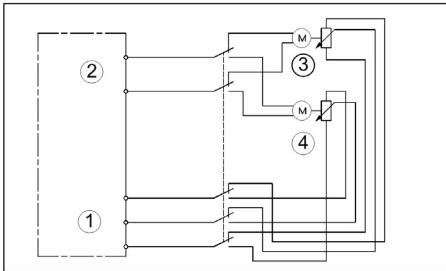
Fig. 9-27 switching from oil motor to gas motor
