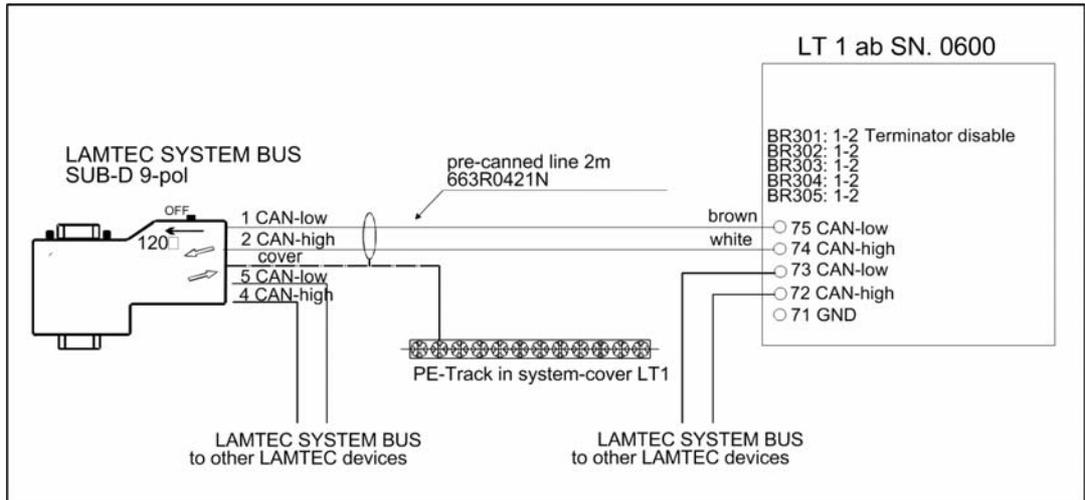
Fig. 9-16 LSB connection ETAMATIC - LT1 - other LAMTEC devices
