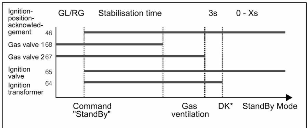
Fig. 8-5 Sequence at gas operation
