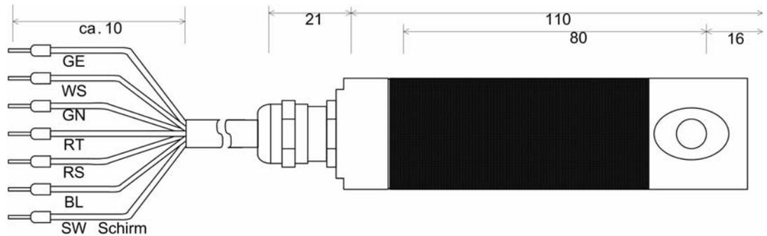
Fig. 9-33 Flame sensor FFS06 IR / VU
