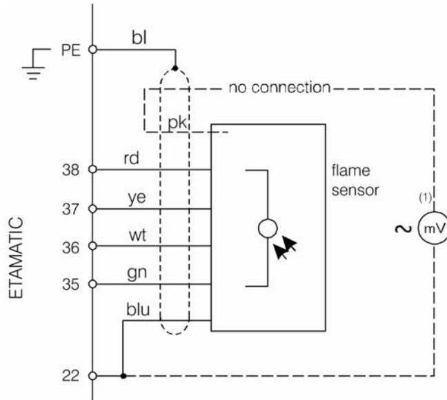
Fig. 9-9 Connection flame monitor
