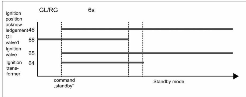
Fig. 8-6 Sequence at oil operation
