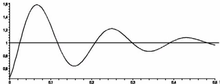
Fig. 8-2 controller operation with I-term too high
