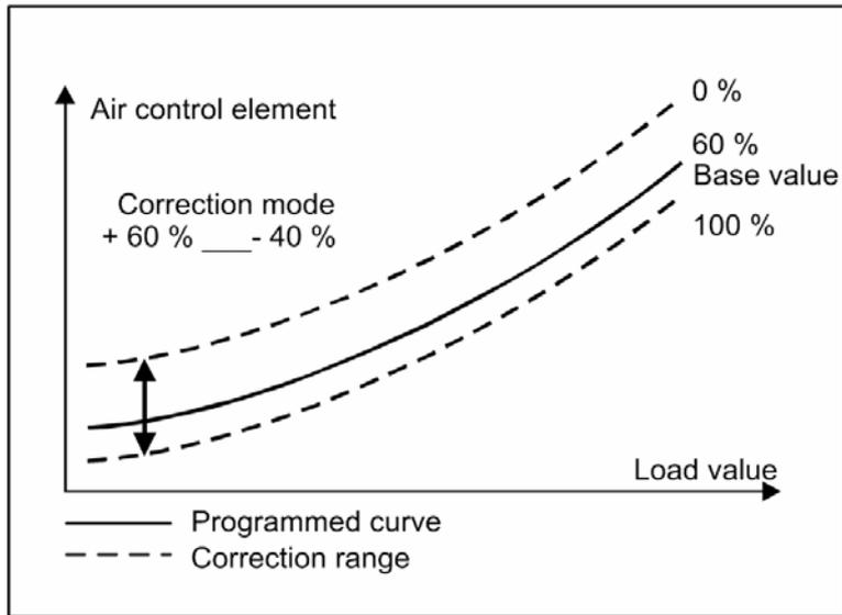
Fig. 6-2 Correction to the setpoint
