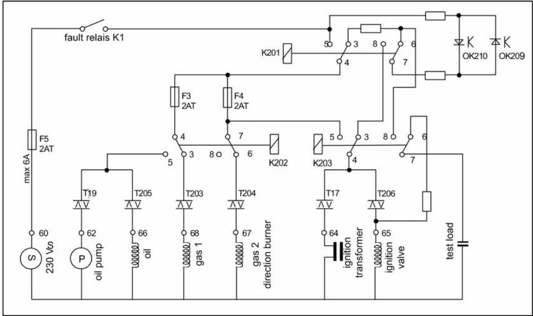
Fig. 9-21 Internal connecting diagram of the control outputs
