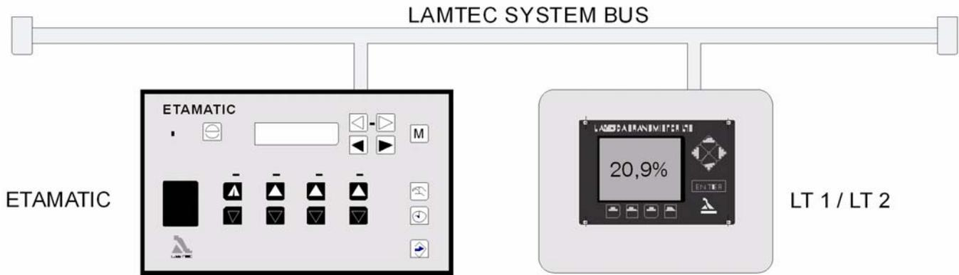
Fig. 6-1 Connection to the O<sub>2</sub> measuring device via LAMTEC SYSTEM BUS
