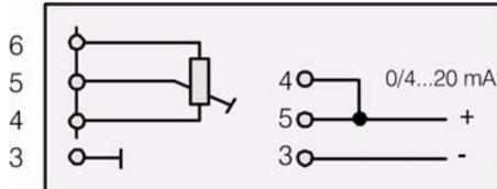
Where a three-point step signal from the firing-rate controller is used as firing-rate input, you must connect the contacts instead of the potentiometer of the firing-rate:
