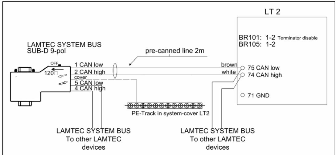
Fig. 9-13 LSB connection ETAMATIC - LT2 - other LAMTEC devices
