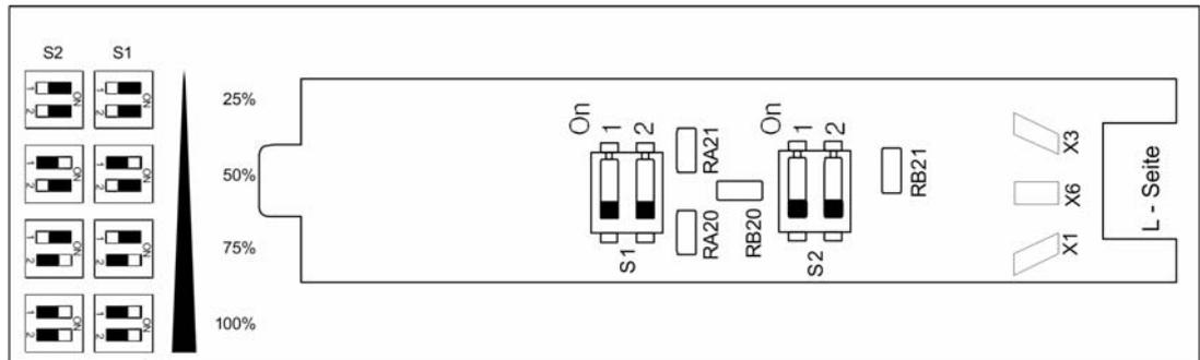
Fig. 9-2 FFS06 There is no sensitivity switch for flame scanner type FFS 06-UV
