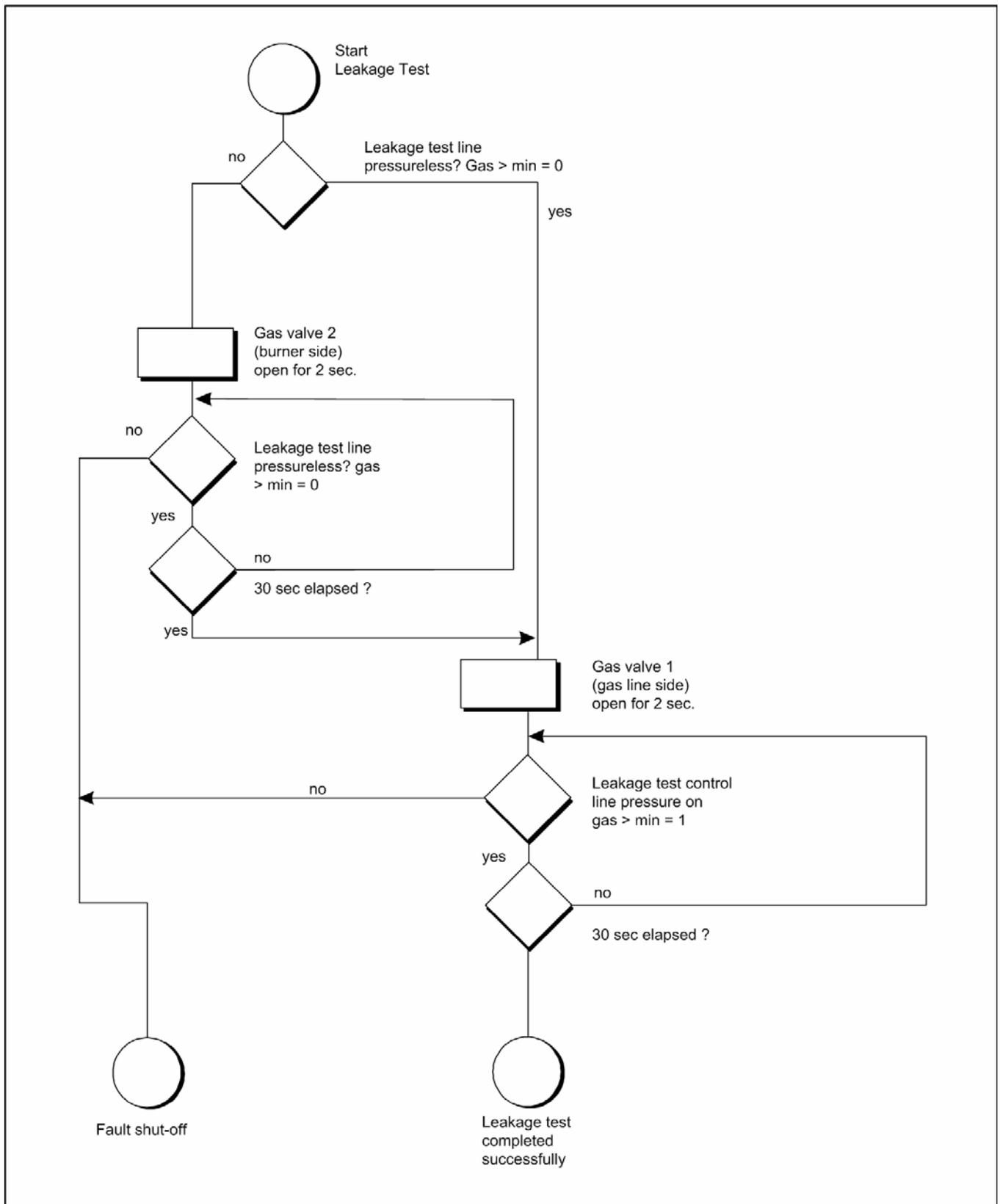
Fig. 8-4 Flow chart leakage test
