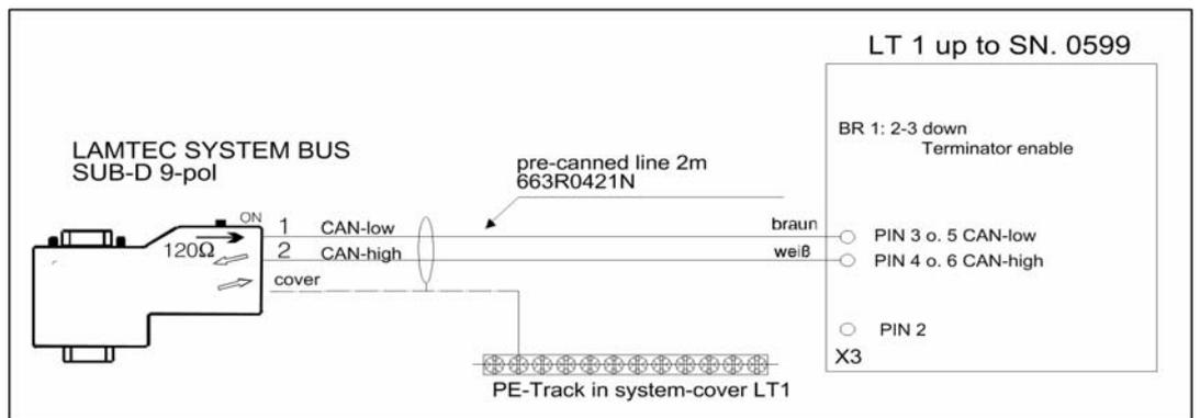
Fig. 9-15 LSB connection ETAMATIC to LT1 up to SN.: 0599
