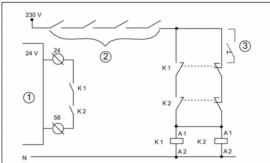
Fig. 9-22 Example: safety interlock chain wiring via 230 V
