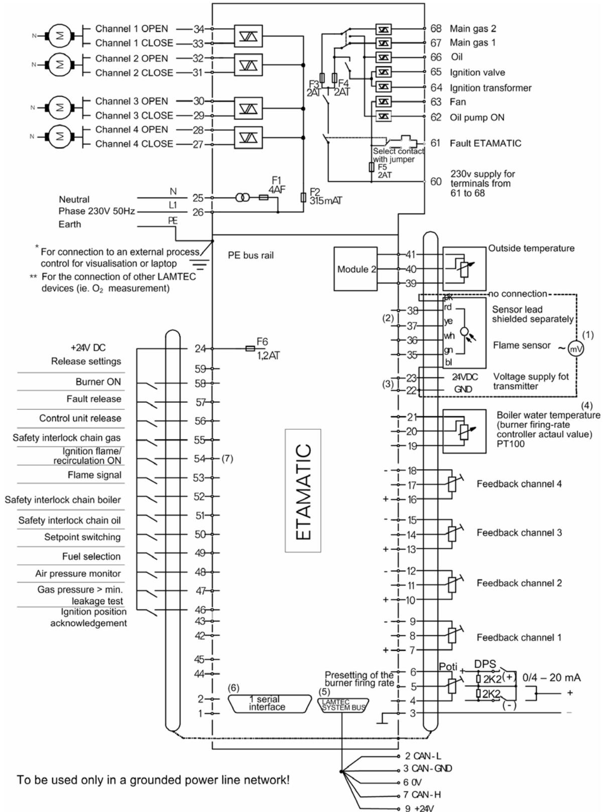
Fig. 9-7 ETAMATIC wiring diagram with ignition flame monitoring
