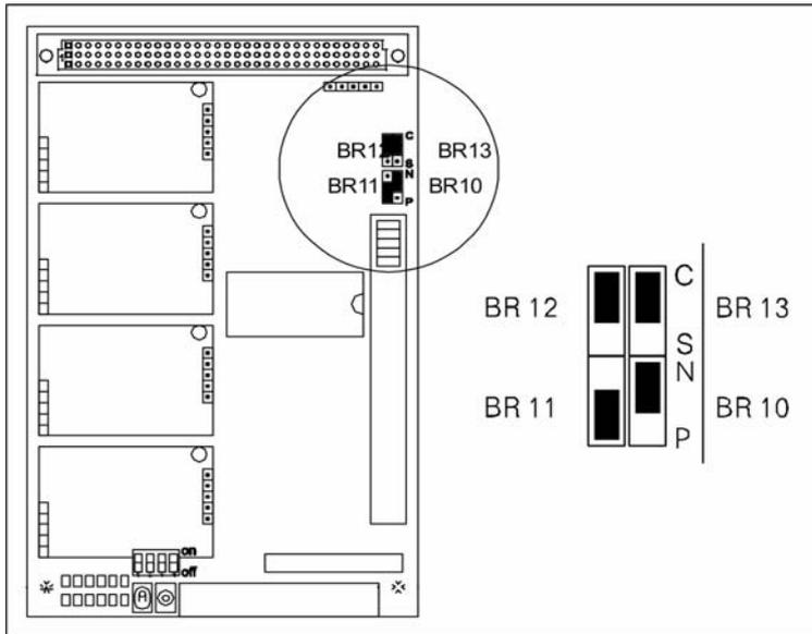
Fig. 9-11 Configuration of the processor board LT1 / LT2 to LAMTEC SYSTEM BUS (LSB)
