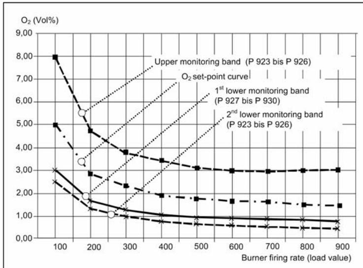
You can set the monitoring bands' parameters for 2 fuels, oil/gas, as a function of fuel. The permitted deviation is calculated as a percentage of the setpoint. You can specify two separate percentage values for base load and full load. The section between is interpolated linearly.
