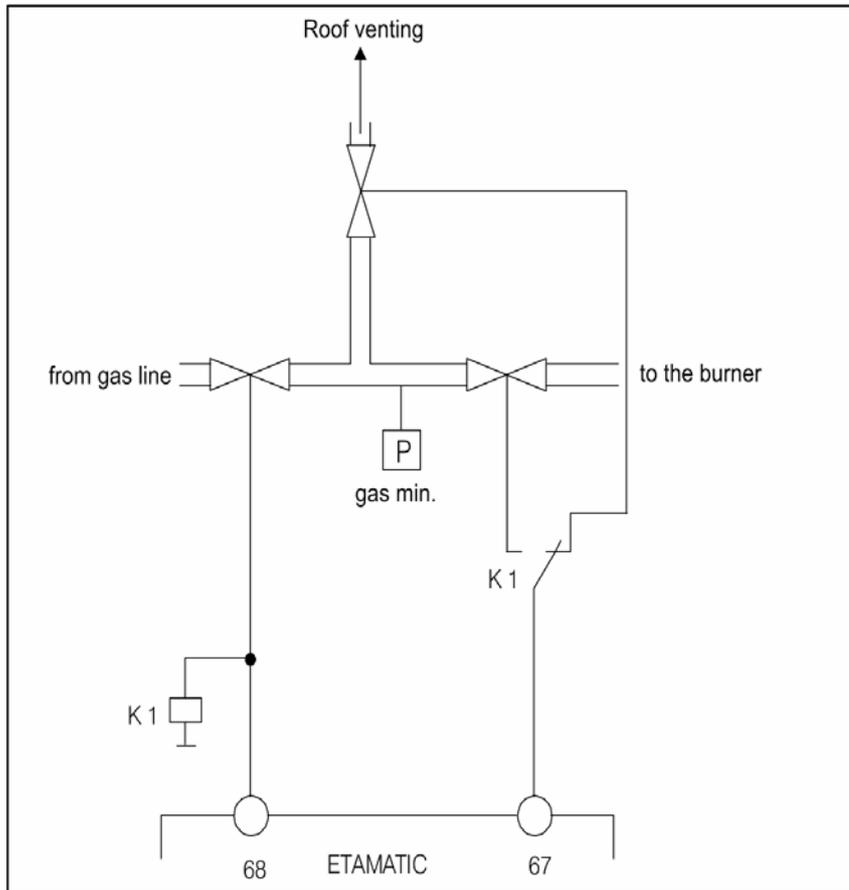
Fig. 9-23 Suggested wiring for venting the gas line over the roof in conjunction with the ETAMATIC
