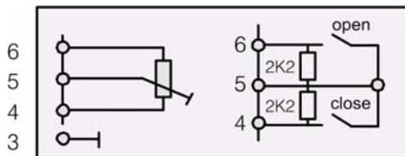
Where a 4-20mA unit shall be supplied with 24V (e.g. a passive steam pressure controller).
