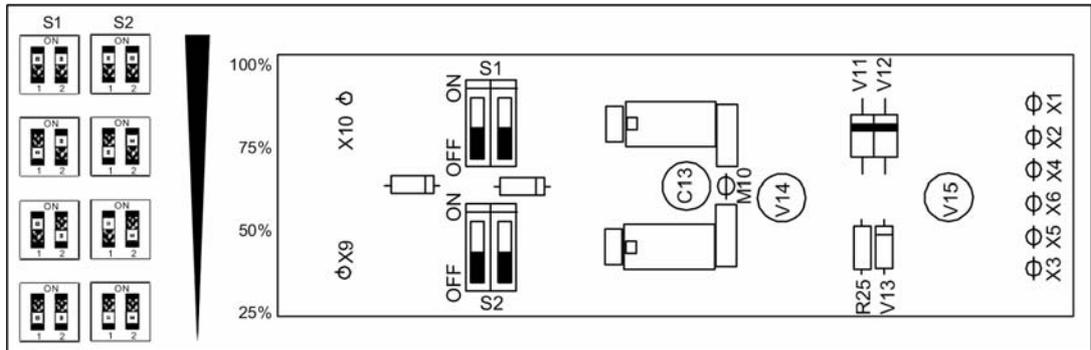
Fig. 9-1 FFS 05 Adjusting the flame sensitivity - factory settings IR 50% UV 100%
