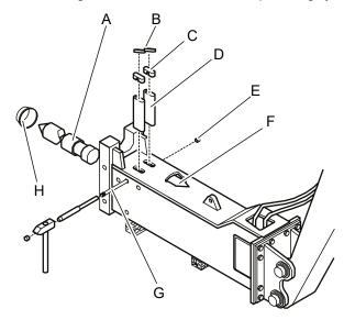
Wiper installed (only hydraulic breakers with DustProtector):
