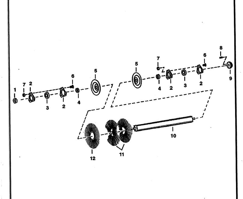
NOTE: To change from Flat Brush Sections to Zig Zag Sections all sections must be changed. 6646703 spacers are not used with Zig Zag Sections.
