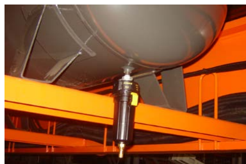
Fig. 7: Dreno / Dreno / Drain / Drain
