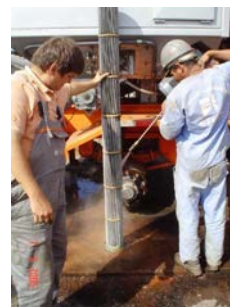
Fig. 4: Lavagem das mangas com jato de água e vassoura / Washing the bags by spraying water and a broom
