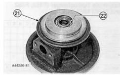
14. Use Tool (G) to remove ring (22). Remove shroud (21) from the cartridge housing.
