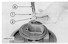
4. Install bearing (2) in the cartridge housing with the short dye mark up
