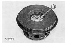
10. Remove deflector (14) and the ring from the cartridge housing.
