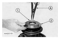
**4.** Put shroud (2) in position on the cartridge housing, and install ring (1) to hold the shroud.
