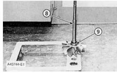
6. Remove seal ring (9) from turbine shaft (8).
