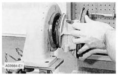
**18.** Install the turbine housing on Tool (E). Put the cartridge assembly in position in the turbine housing. Make sure the marks on the housings are in alignment with each other. Put **5P3931 Anti-Seize Compound** on the threads of the "V" clamp that holds the cartridge assembly to the turbine housing. Install the "V" clamp and tighten the bolt to a torque of **13.6 ± 1.1 N·m (120 ± 10 lb in)**.
