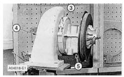
2. Remove "V" clamp (3). Remove cartridge housing (5) from turbine housing (4).
