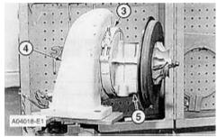
2. Remove "V" clamp (3). Remove the cartridge housing (5) from the turbine housing (4).
