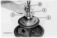
5. Install bearing (5) in the cartridge housing with the short dye mark up. Install sleeve (4).
