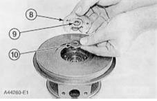
8. Install ring (10), sleeve (9) and bearing (8) in the cartridge housing.
