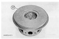
**12.** Use Tool (F), and remove the ring that holds bearing (17) in position. Remove bearing (17), and put a long dye mark on the top face of the bearing.
