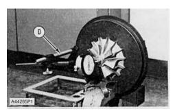
**17.** Put cartridge housing in a vise as shown. Check the shaft end play with Tool (D). The end play must be **0.114 ± 0.038 mm (.0045 ± .0015 in).** If the shaft end play is not the correct dimension, the inside parts of the cartridge housing must be checked for too much wear. See Turbocharger (Schwitzer 4MF AND 4MFW) in Specifications.
