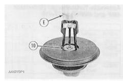
8. Remove insert (10) with Tool (E).
