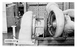
**19.** Install the compressor housing to the cartridge assembly. Install the "V" clamp that holds the compressor housing to the cartridge housing and tighten bolt to a torque of **13.6 ± 1.1 N·m (120 ± 10 lb in)**.
