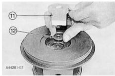
9. Install ring (12) and deflector (11) in the cartridge housing.
