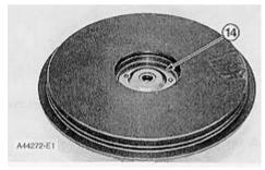
10. Remove deflector (14) and the ring from the cartridge housing.
