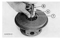
**7.** Turn the cartridge assembly over, and install bearing (7) with the long dye mark up. Use Tool (B), and install ring (6) to hold the bearing in position.
