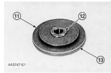
**9.** Remove O-ring seal (13) and sleeve (12) from insert (11). Remove the seal rings from sleeve (12).
