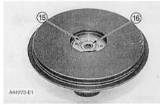
11. Remove bearing (15), sleeve (16) and the ring from the cartridge housing.
