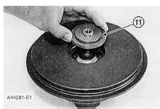
**12.** Install insert (11) in the cartridge housing. Use Tool (B) and install the ring to hold the insert in position.
