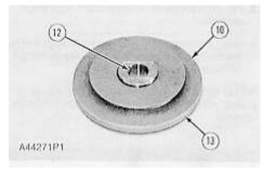
9. Remove O-ring seal (13) and sleeve (12) from insert (10). Remove the seal rings from sleeve (12).
