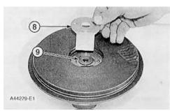
8. Install ring (9) and deflector (8) in the cartridge housing.
