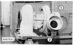
**1.** Install turbocharger in Tool (A). Put marks on the three housings of the turbocharger for correct installation and alignment at assembly. Remove "V" clamp (2) and compressor housing (1).
