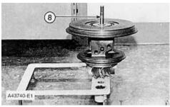
5. Remove turbine shaft (8) from the cartridge housing.
