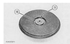
7. Use Tool (D) and remove ring (11) that holds insert (10) in the cartridge housing.
