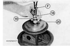
13. Turn the cartridge assembly over. Use Tool (F), and remove ring (18). Remove sleeve (19) and bearing (20) from the cartridge housing. Put a short dye mark on the top face of bearing (20).
