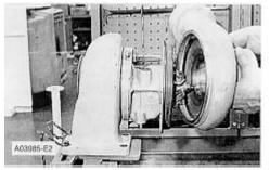
20. Install the compressor housing to the cartridge assembly. Install the "V" clamp that holds the compressor housing to the cartridge housing and tighten the bolt to a torque of  $14 \pm 3 \text{ N} \cdot \text{m}$  (10 ± 2 lb ft).
