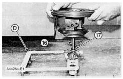
**14.** Install seal ring (17) on turbine shaft (16).
