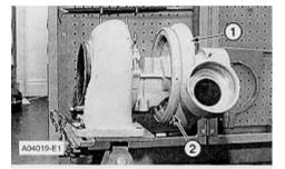
1. Install the turbocharger in Tool (A). Put alignment marks on the three housings of the turbocharger for correct installation and alignment at ial Green assembly. Remove "V" clamp (2) and compress housing (1).
