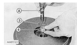
ring (4) with . 6. Turn the cartridge assembly over and install bearing (4) with the long dye mark up. Use Tool (A) and install ring (3) to hold the bearing in pillar Inc. position.
