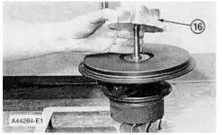
15. To install compressor wheel (16) on the turbine shaft, make reference to Turbocharger Impeller Installation, Schwitzer only in Specifications.
