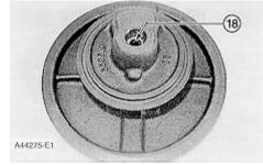
**13.** Turn the cartridge assembly over. Use Tool (F) and remove the ring that holds bearing (18) in position. Remove bearing (18) from the cartridge housing. Put a short dye mark on the top face of bearing (18).
