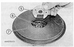
**7.** Install ring (7), sleeve (6) and bearing (5) in the cartridge housing.
