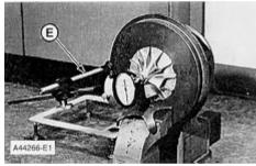
18. Put the cartridge housing in a vise as shown. Check the shaft end play with Tool (E). The end play must be 0.114 ± 0.038 mm (.0045 ± .0015 in). If the shaft end play is not the correct dimension, the inside parts of the cartridge housing must be check for too much wear. See Turbocharger (F452, F552 and F555) in Specifications section. erpillar Inc
