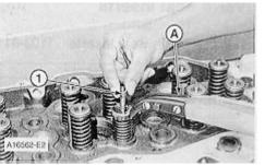
2. Put the springs in compression with Tool (A).
