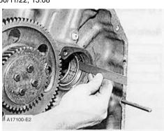
2. Install the front camshaft bearing with Tool (A) until it is 7.34 ± 0.10 mm (.289 ±,004 in) from the machined surface on the front of the cylinder block as shown.
