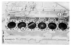
2. Install six 3/8" -16 NC forcing screws (3) in the spacer plate. Tighten the screws evenly until the plate is free of the dowels on the cylinder head.
