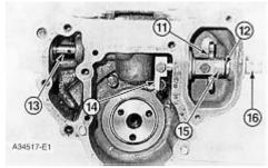
7. Remove the bolts from levers (14) and (11). Remove shaft (16), lever (14), lever (11), bearing (15) and spring washer (12).
