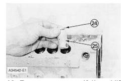
**13.** Remove spacers (24) and lifters (25) from the injection pump housing. Put identification on each of the spacers and lifters as to their location in the pump housing.
