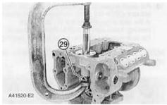
20. Install pinion gear (29) in the pump housing. Use an 11/16 socket and a "C" clamp with a minimum opening of 22.9 cm (9 inches) and install pinion gear (29) until the pump drive makes contact with the shoulder of the pinion gear shaft.
