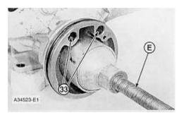
18. Remove the rack bearings from locations (33).
