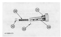
21. Install spring (30) and piston (32) in valve body (34). Install pin (33). Install seal (31).
