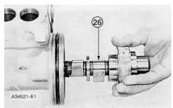
14. Remove camshaft (26) from the pump housing.
