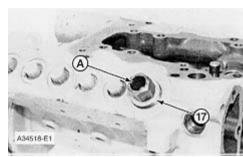
9. Remove the felt washer from bushing (17). Remove bushing (17) from each of the injection pumps with Tool (A).
