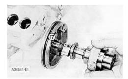
14. Put clean engine oil on the camshaft bearings and on camshaft (17). Install camshaft (17) as shown.
