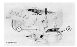
1. Remove bolts (1) from rear cover (2). Remove cover (2) and gasket.
