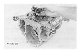
19. Install idler gear (27) on the shaft. Put drive gear (28) in position with the bevel side of the gear down. Make sure the teeth of the idler gear and drive gear are in alignment and install the pump cover.
