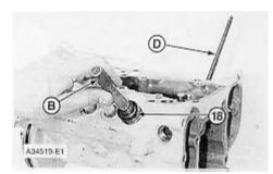
**10.** Install Tool (D) in the pump housing with the square end down (end with taper will be up). Hold the racks against Tool (D) and remove each of the injection pumps (18) with Tool (B). For more details, see Remove Fuel Injection Pumps.
