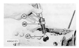
28. Put the space in gear segment (47) alignment with the groove in pump barrel (46). Put the injection pump straight down into the housing bore with the space in gear segment (47) engaged with the pin in the lifter and the groove in barrel (36) engaged with the dowel in the pump housing. Use Tool (H) to install the pumps.
