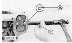
13. Install seal (16) with Tool (E). Install the seal until it is even with the surface of the pump housing and with the lip toward the outside as shown.
