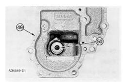
**32.** Install bearing (50) in rear cover (49) with Tool (J).
