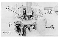
5. Remove idler gear (7). Remove pinion gear assembly (9) from the pump housing with a soft hammer as shown. Remove drive gear (8).
