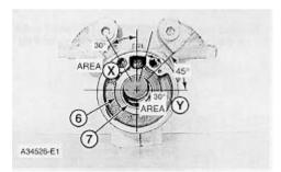
5. Install the camshaft front bearing (7) with Tool (B). Install the bearing until it is 1.02 ± 0.51 mm (.04 ± .02 in) from front surface (6) of the pump housing.
