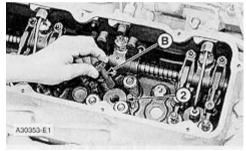
Pillar Inc. 4. Loosen adapters (2) with the correct Tool (B) or (C). Remove the adapters from the cylinder head.
