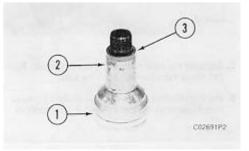
2. Put 5P3931 Anti-Seize Compound on the threads of adapter (2). Install adapter (2) and gasket (3) in the cylinder head. Tighten the adapters to the correct torque as follows:
