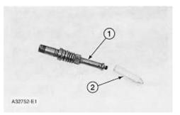
2. Install nozzle (2) on valve body (1) finger tight.
