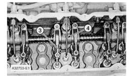
**3.** Install the fuel injection value in direct injection adapter (3). Make sure the grooves (serrations) on value body (1) are in alignment with the grooves (serration) in adapter (3).
