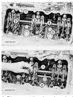
1. Disconnect the glow plug wire from the glow plug and clip (2) from fuel line (1). Remove line (1) with Tool (A).
