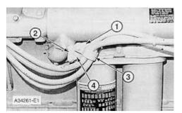
1. Remove the bolt from clamp (3). Reposition the clamp and hoses. Remove cover (4).
