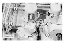
1. Remove bolts and clamps (2) that hold service meter (1) to tachometer drive (4). Remove service meter (1).
