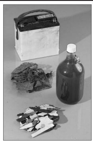
S crap lead-acid batteries are disassembled in a ventilated battery breaker, where the lead, plastic and acid are safely separated.
