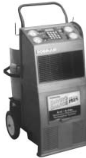
Typical Air Conditioner Refrigerant Unit
