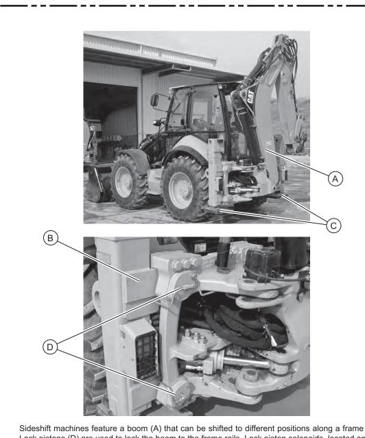
Sideshift machines feature a boom (A) that can be shifted to different positions along a frame (B). Lock pistons (D) are used to lock the boom to the frame rails. Lock piston solenoids, located on the backhoe valve outlet manifold, actuate the lock pistons.
