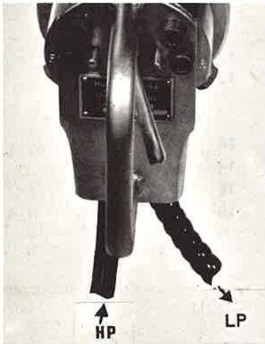
1. Lever center: Fluid circulates in system.
