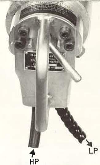
LEVER RIGHT POS. 3 – RETRACT PLUG
