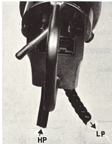
2. Lever left: Fluid forces plug forward.
