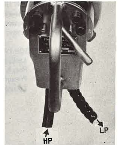
3. Lever right: Fluid forces plug back.
