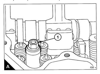
**Caution:** Before installation ensure that the injector sleeve and its bore in the cylinder head are clean and free from oil, dirt and sealant.
