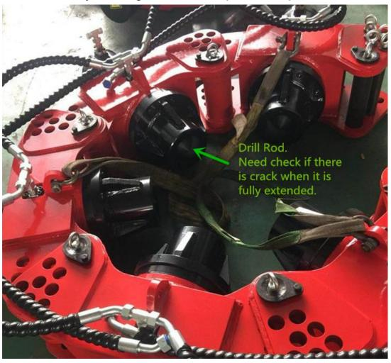
3. Hydraulic parts (oil cylinder, oil hose and joints.) If there is any damage, please replace immediately.
