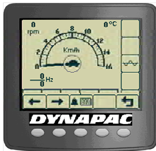
Figure. The display shows the selection in the middle (tortoise or rabbit).
