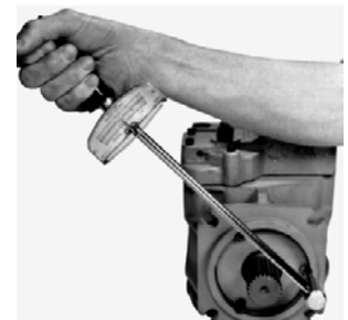
Torque Retainer Screw
