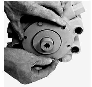
Install Screws and Cover Retainer
