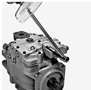
90000334 Torque PCP Valve Screws
