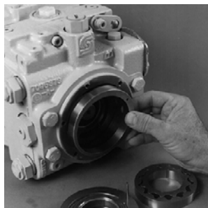
Install Gerotor Assembly Outer Ring
