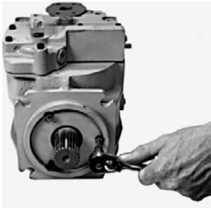
90000270 Remove Screws Holding Retainer Plate and Seal Carrier
