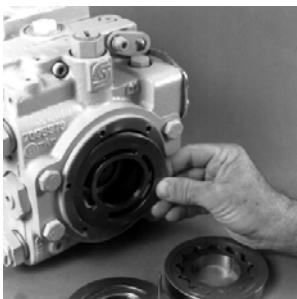
Install Inner Port Plate
