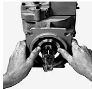
Install Seal Carrier
