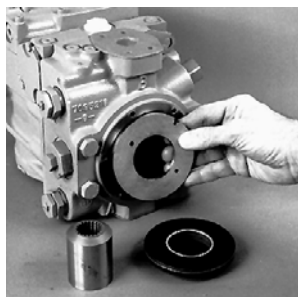
Install Spacer Plate (Intermediate production only)
