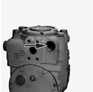
Charge Pump Inlet
