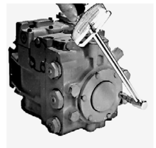
90000295 Torque Retainer Screws
