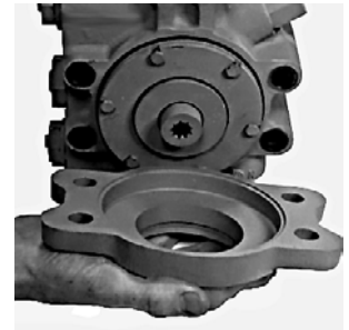
Install Auxiliary Pad Adapter
