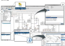
3 > Part use shows where the corresponding parts are installed in the machine and enables you to jump to the parts catalogue.
