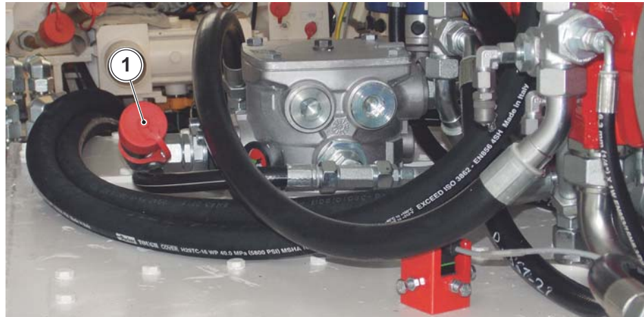
Figure IV - 9: Tank filling connection
