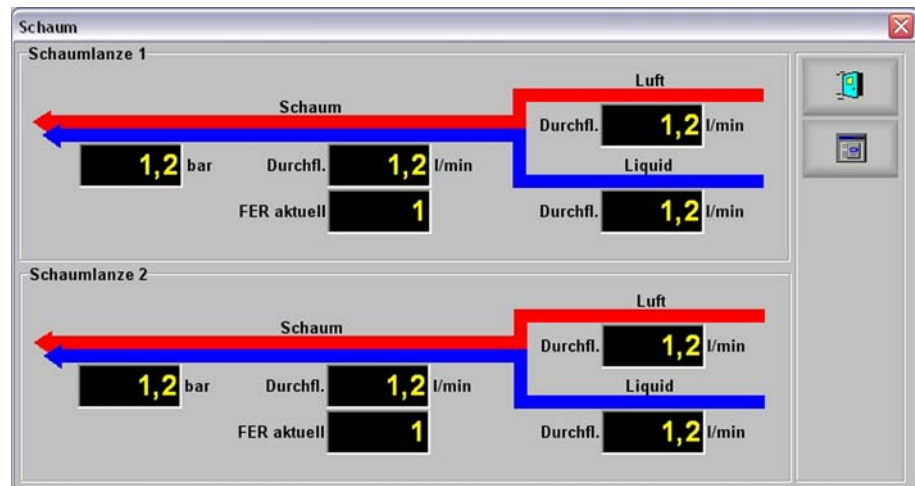
"Infocentre foam generator" screen
