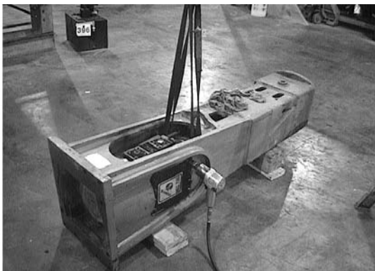
Fig. 28 – Unloading & Removing Side Shocks
