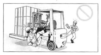
Do not get on/off a forklift if it is moving. When getting on/off a forklift, confirm that it is stationary in the first place and get on/off as per correct steps. Tread on the step and hold the handrail to support the body when getting on/off. In addition, the steps shall be clean.
