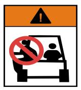
It is not safe to load passengers on the forklift because the vehicle body vibrates greatly in case of bumpy roads. Especially, because of small turning radius, persons are easy to be swung externally.
