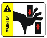
Never put your hand or foot in the mast or gap connecting the mast; otherwise, once the mast moves, injuries may be caused.
