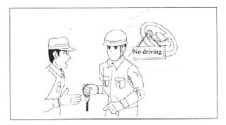
Do not drive the vehicle that has abnormality during the spot inspection until it is repaired by the shop. Affix a label saying **No Driving** and take out the key. Report the situation to the manager and authorize him to repair it.
