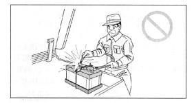
Do not allow any metal to directly contact the battery terminals – and + to short it. A slack terminal – may spark due to poor connection, which may cause an explosion. Terminals must be securely tightened. After removing the battery, confirm its terminals – and +. Do not connect them inversely when re-installing the battery.
