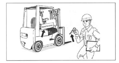
The key of a faulty vehicle must be taken out and a sign saying NO USE shall be affixed.
