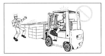
Drive carefully when loading/unloading long and wide cargo. Lift or lower it slowly and especially do not collide it with other cargo.
