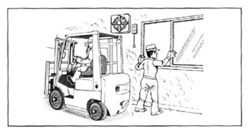
In an enclosed warehouse, waste gas emitted from the engine operation may cause toxic hazard and deaths under the worst condition. Open windows and doors during production and turn on the ventilator for ventilation. In case of operation in the warehouse for long, ventilation capability must be researched in details.
