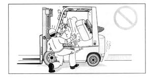
The engine oil may be of high temperature and pressure after vehicle operation. Oil drain and filter element replacement under this condition will cause high temperature engine oil to be sprayed out, causing scald easily.
