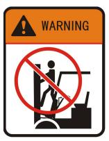
It is hazardous to use the forklift body as the step and mast as the ladder. Unintentional operation of the control stick may cause an unpredictable movement of the mast and the person may be crushed between the mast and body, causing major accidents.
