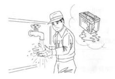
The electrolyte of the battery contains the dilute sulphuric acid that corrodes the clothes and skin. If the electrolyte contacts the clothes or skin, flush it immediately with much water.
