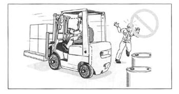
Face the rear when driving backwards and start driving after confirming the rear condition directly. Do not depend on only rear-view mirrors and reversing buzzer.
