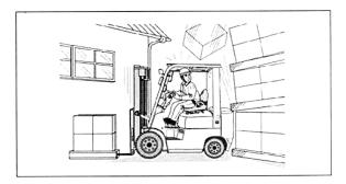
An overhear guard is used to protect the driver's head from being impacted by fallen objects. However, it is not available to resist the impact of all kinds of objects.
