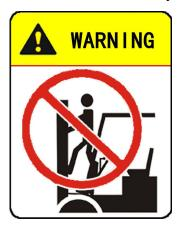
It is dangerous to use the forklift's body as the step and mast as a ladder. Unintentional contact with the control handle may cause unpredictable mast movement and the person may be crushed between the mast and vehicle body, causing a major accident.
