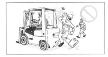
The antifreeze is of high temperature and pressure after vehicle operation. Do not open the water tank cover under this condition; otherwise, high temperature antifreeze may be sprayed out, causing scald easily.
