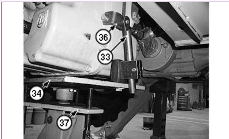
TX1017775A-UN: Low Lift Transmission Jack and Mounting Bracket (left side)
