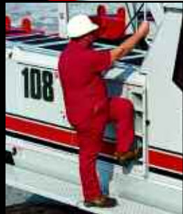
Wide-opening doors (upper left), two upper access ladders with hand-rails (left) and fold-up treadmember steps prove that access is the name of the game on the 108 H5.
