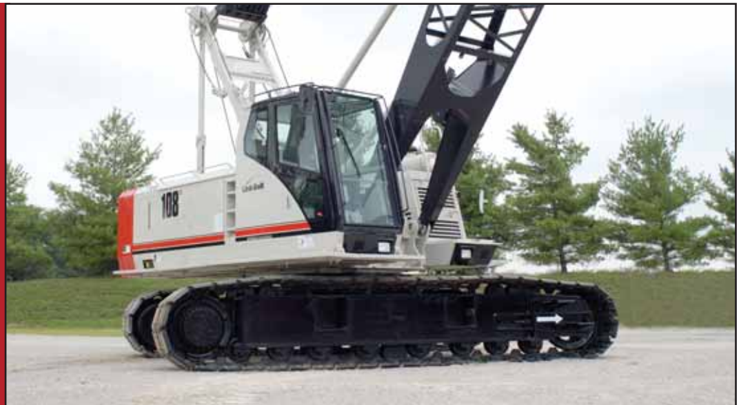
The 108 H5 has standard toe plates, which enable blocked over-end capacities, challenging higher rated capacity cranes.
