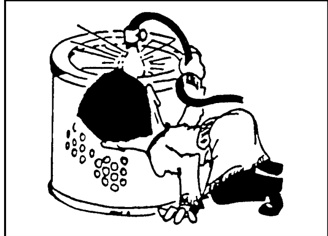
Figure 2-9 Inspecting the air cleaner element.
