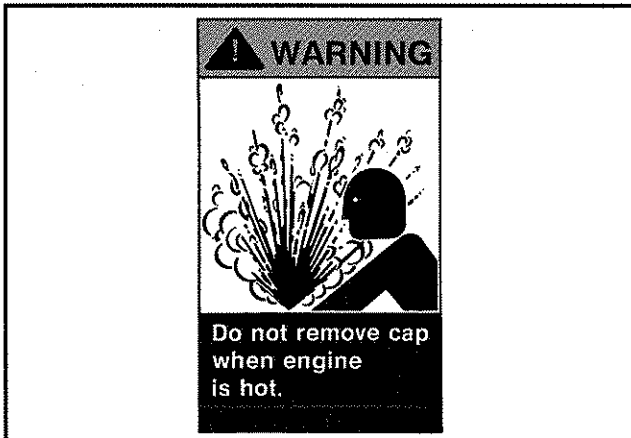
Figure 2-5 Allow engine to cool before removing the fill cap.
