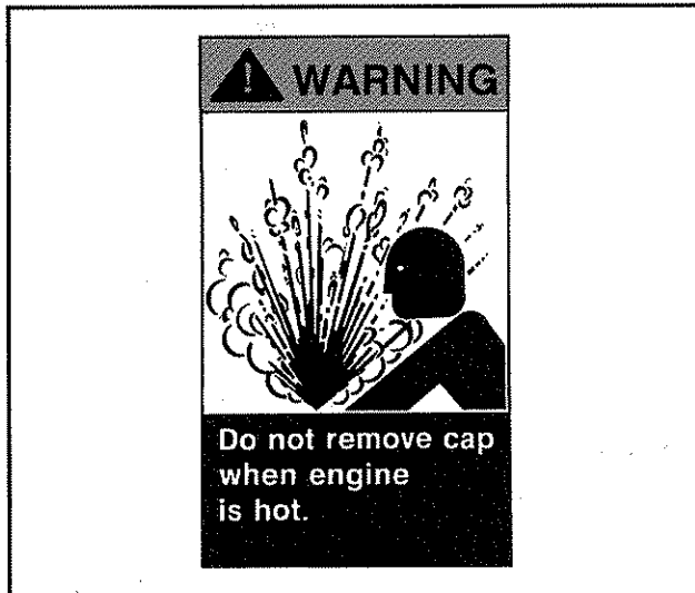
Figure 1-23 Allow engine to cool before removing the radiator cap.
