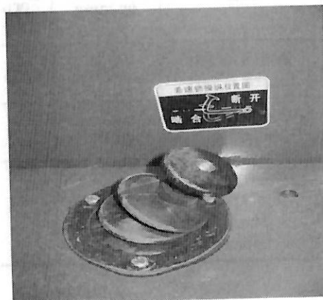
Fig. 3-36 Differential lock operation
