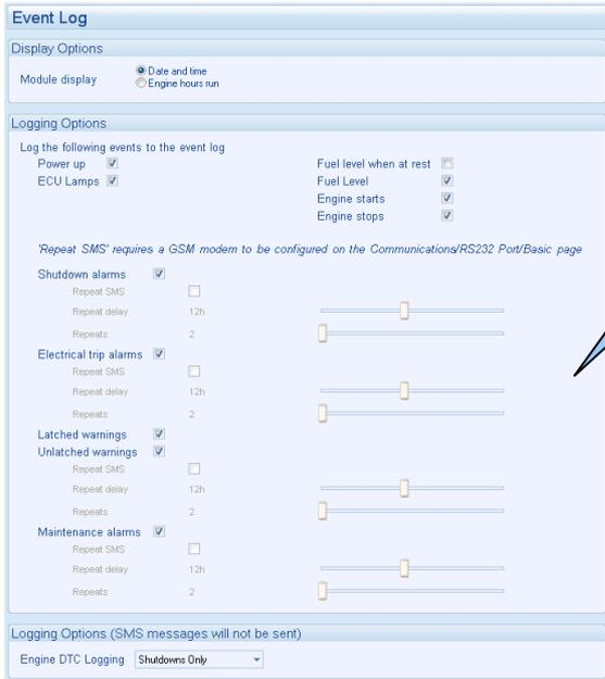
Example showing the possible configuration of the event log (DSE Configuration Suite Software).
