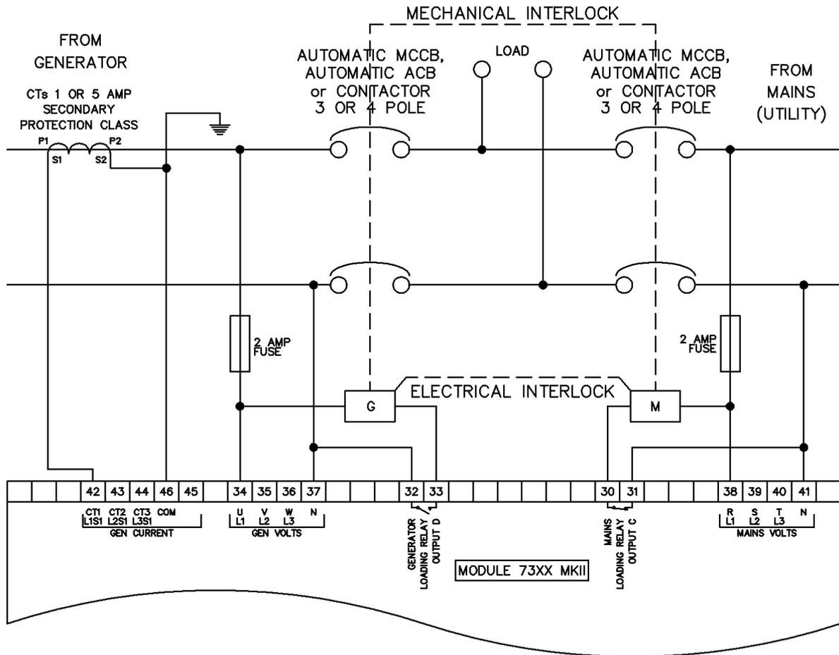
3.4.3 SINGLE PHASE (L1 & L2) 3 WIRE WITH RESTRICTED EARTH FAULT
