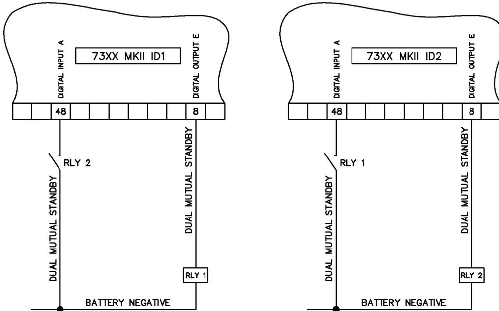
In case of set 1 failure, the output activates and energises the external relay RLY1 to call for the second set to start.
