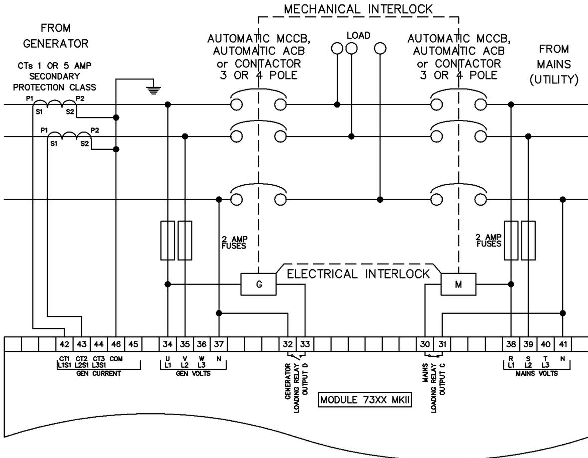
3.4.9 2 PHASE (L1 & L3) 3 WIRE WITH RESTRICTED EARTH FAULT
