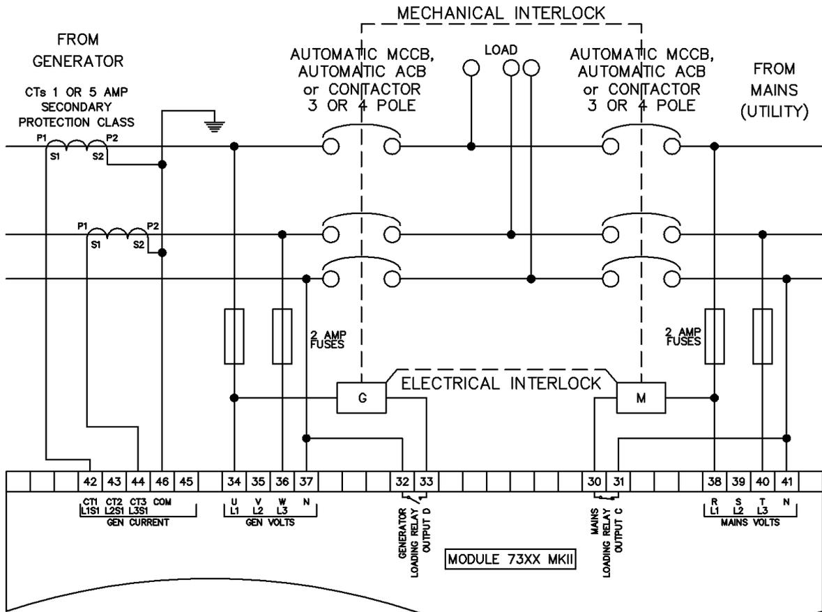
3.4.7 2 PHASE (L1 & L2) 3 WIRE WITH RESTRICTED EARTH FAULT
