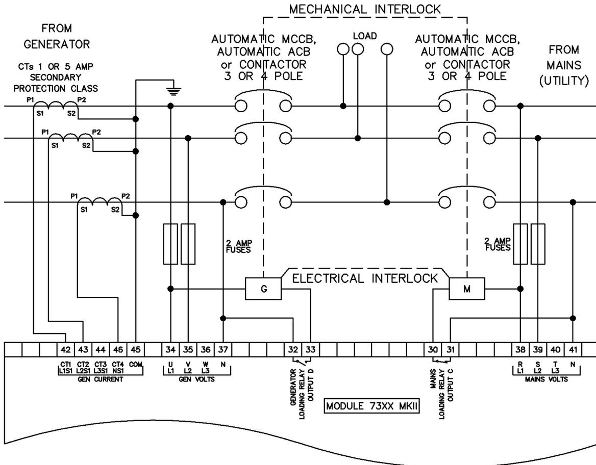
3.4.4 SINGLE PHASE (L1 & L2) 3 WIRE WITHOUT EARTH FAULT
