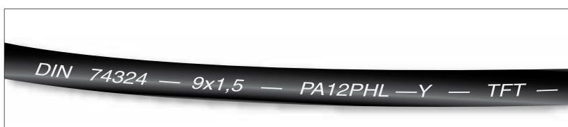
Fig. 51: Engine coolant pipe identifier (size 9 x 1.5; PA12-PHL-Y, printed in white, pipe colour black) ESC-429
