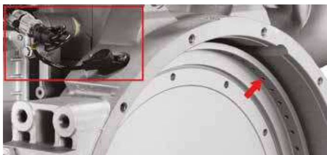
Figure 16: Rpm sensor mounting position
