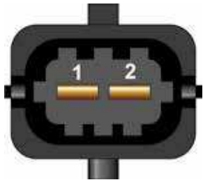
Figure 22: Electrical connections of the camshaft sensor
