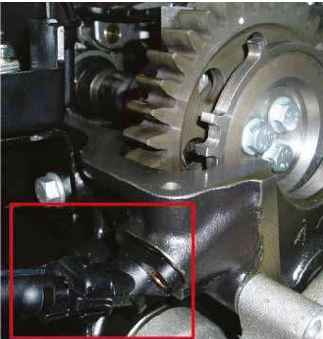
Figure 20: Camshaft rpm sensor mounting position
