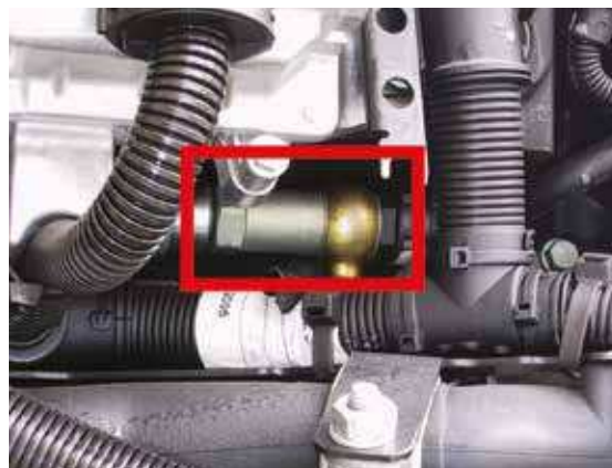
Figure 7: DBV valve in D20 engines
