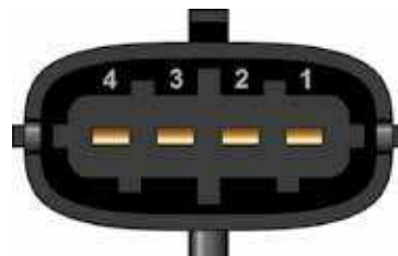
Figure 14: Connections of Bosch intake air pressure sensor (D20)
