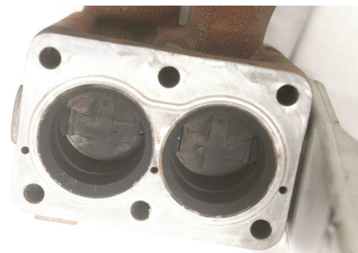
Figure 7. EGR Valves (butterfly)
