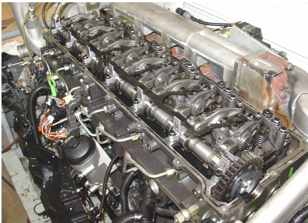
Figure 41. Camshaft and Valvetrain (installed, left rear view)
