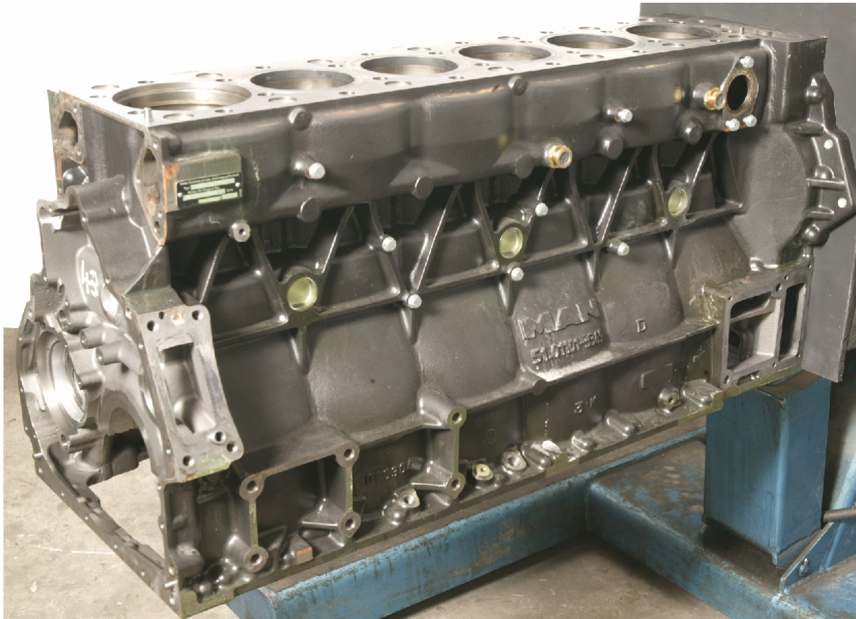
Figure 64. MAN D20 Engine Block (left side view)
