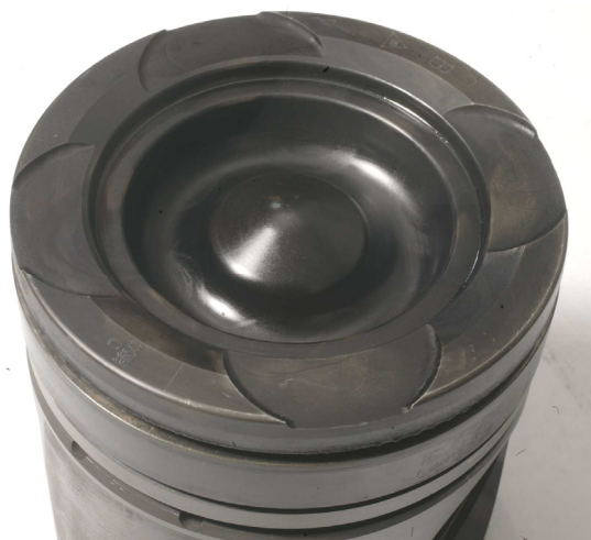
Figure 51. Piston Crown and Valve Pockets
