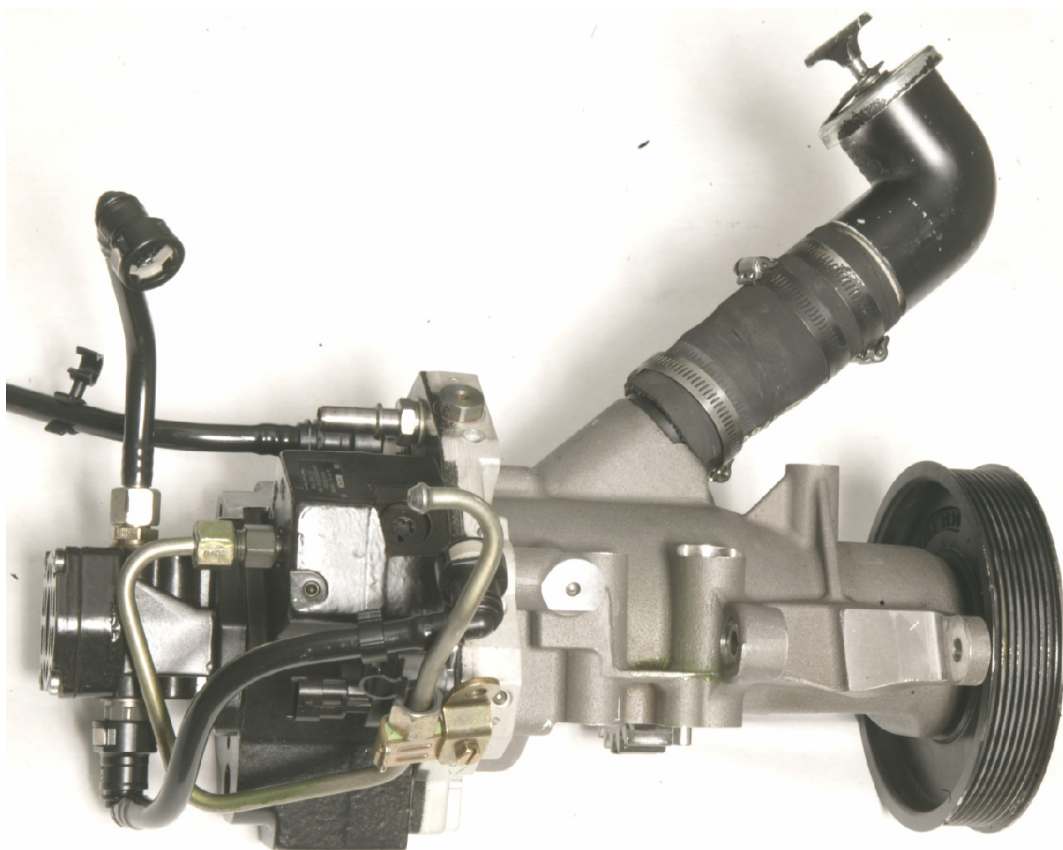
Figure 85. Fuel Supply and High Pressure Pumps, Fuel Manifold/Valve Block, Accessory Drive Pulley and Oil Fill
