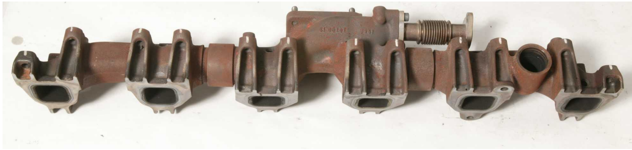
Figure 19. Exhaust Manifold (top view)
