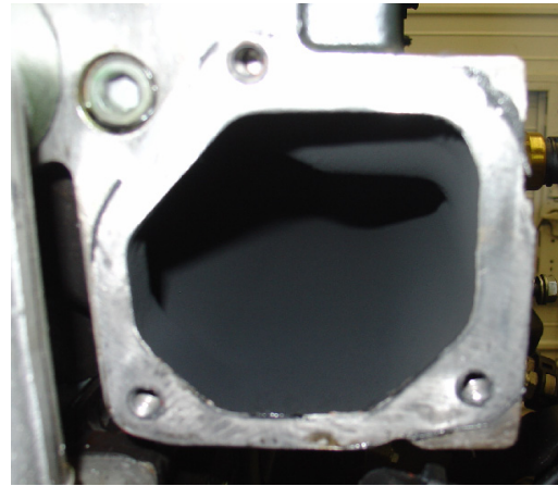
Figure 23. Cylinder Head Intake Manifold Entrance (pipe mount face)
