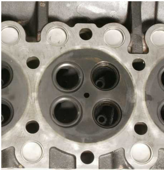
Figure 28. Cylinder Head - Four Valve Arrangement (bottom view)
