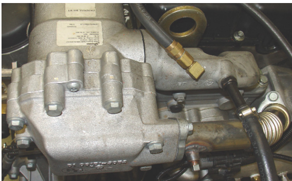
Figure 11. Reed Valve Housing (installed, top)
