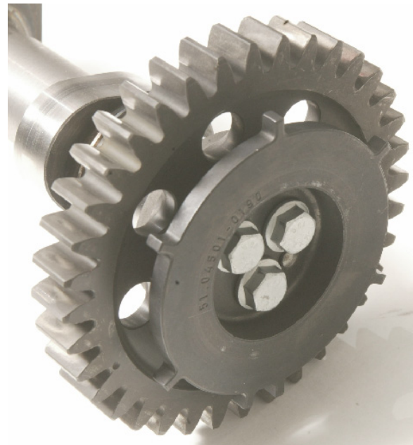
Figure 39. Camshaft Gear and Position Wheel
