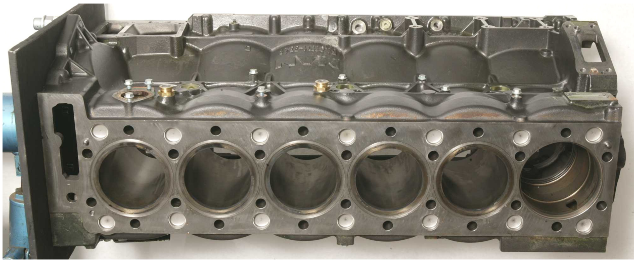
Figure 63. MAN D20 Engine Block (top view)
