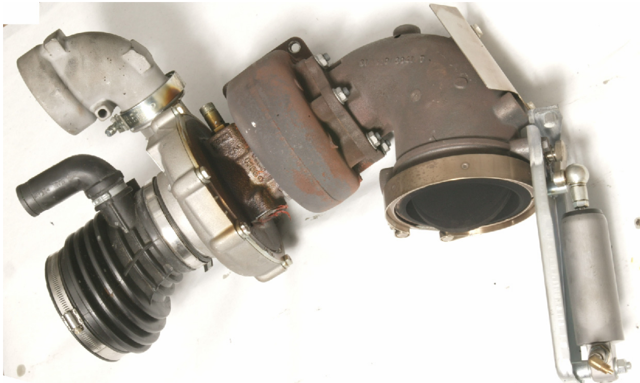
Figure 14. Turbocharger with Inlet Air Connector / CCV Mixer, and Exhaust Brake
