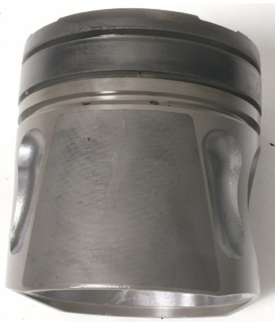
Figure 50. Piston Skirt with Coating
