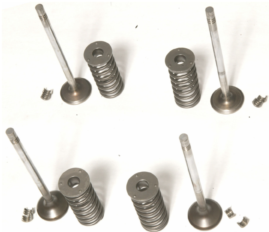
Figure 33. Intake & Exhaust Valves, Springs, Retainers and Keepers
