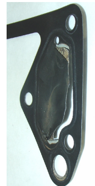
Figure 66. Torn Front Gasket
