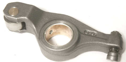
Figure 44. Rocker Arm (bearing view)
