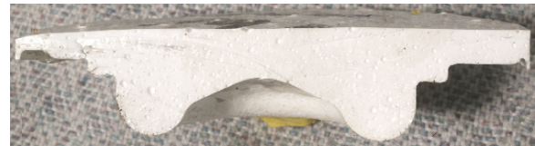
Figure 54. Piston Bowl Mold
