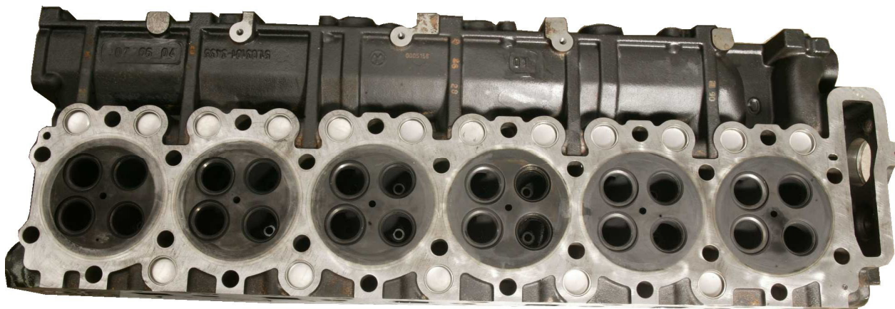
Figure 27. Cylinder Head with Cast-In Intake Manifold (firedeck view)
