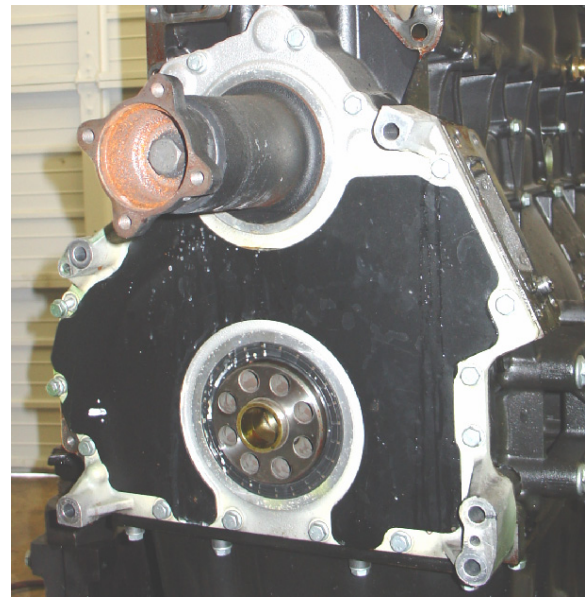
Figure 79. Front Gear Train Cover (installed)
