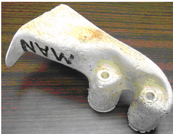
Figure 29. Intake Port Mold (iso view)
