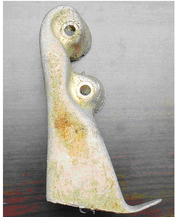
Figure 30. Intake Port Mold (top view)
