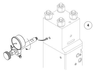
Put in place and screw the inflating tool without touching the control knob.
