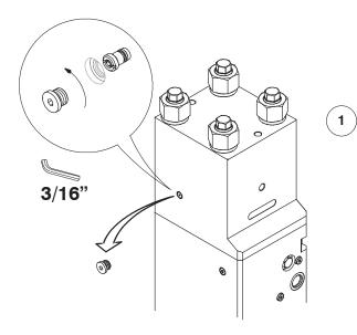
Unscrew the plug with hexagonal key (3/16") and remove it.
