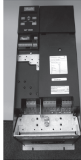
1.VLT 2880-2882 after removal of front cover.
