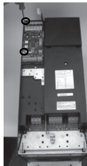
4.Loosen the control card by loosening the two screws with a screwdriver, Torx 10.
