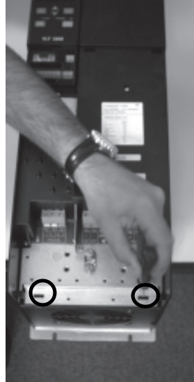
2. Remove the fan by pushing down the two encircled taps.
