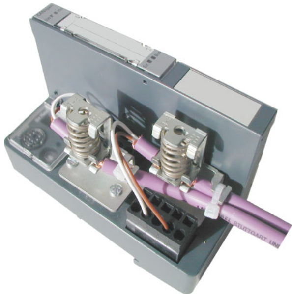
Figure 7: Shielding connection for an XN-GW-CANopen
