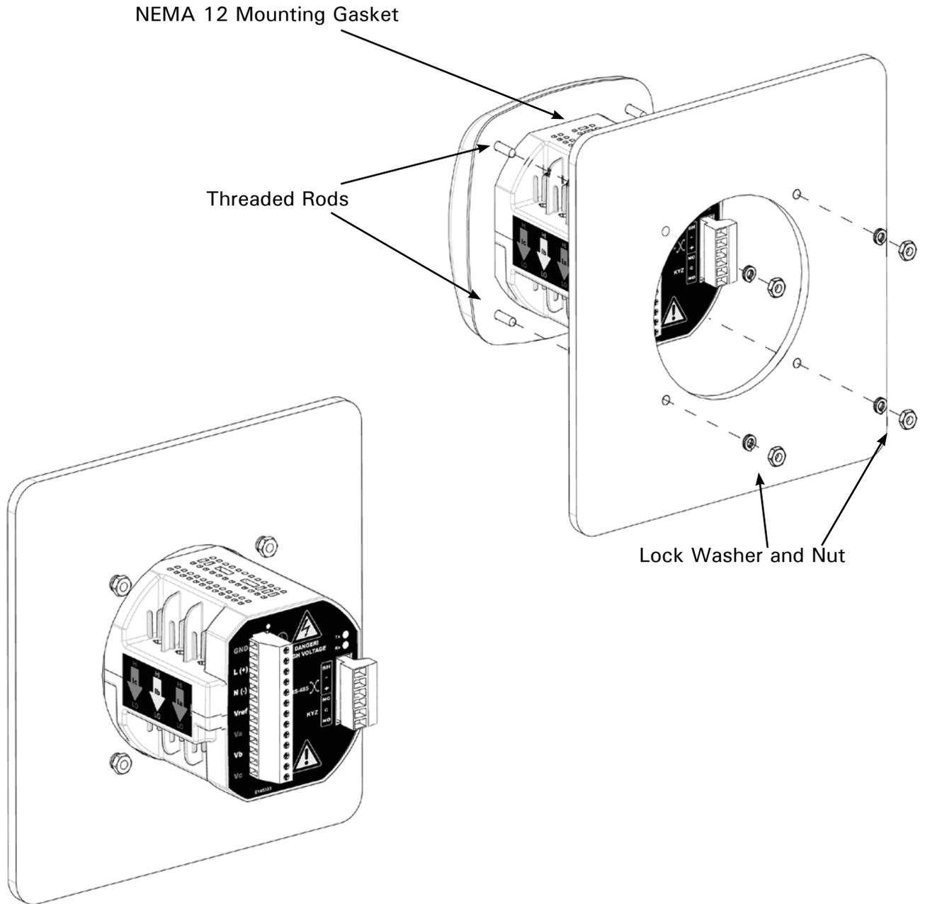
1. Insert 4 threaded rods by hand into the back of the meter. Twist until secure.
