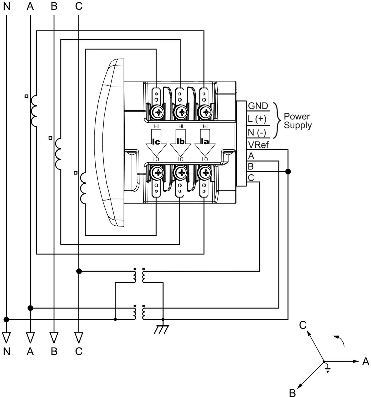
Select: "2.5 EL WYE" (2.5 Element Wye) in Meter Programming setup.
