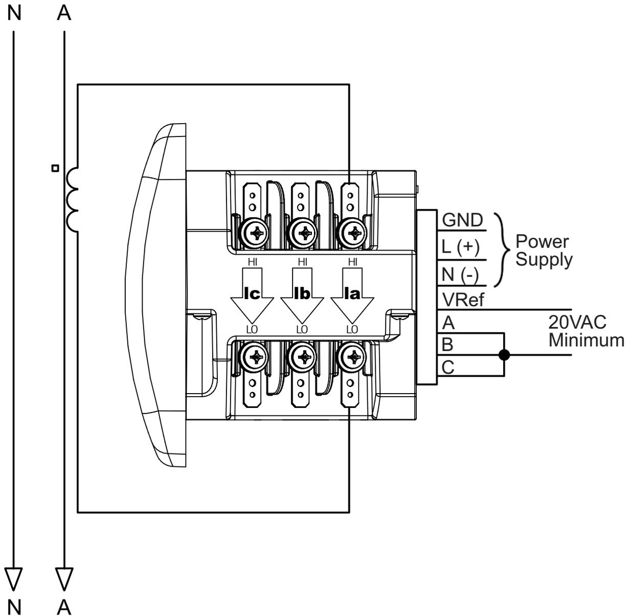
Select: "3 EL WYE" (3 Element Wye) in Meter Programming setup.
