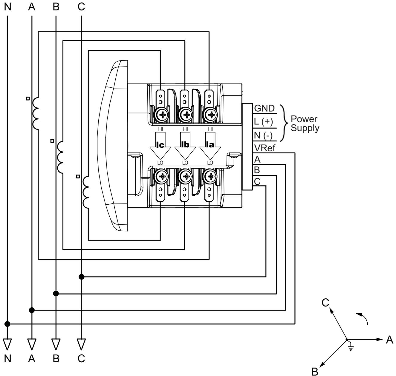
Select: "3 EL WYE" (3 Element Wye) in Meter Programming setup.
