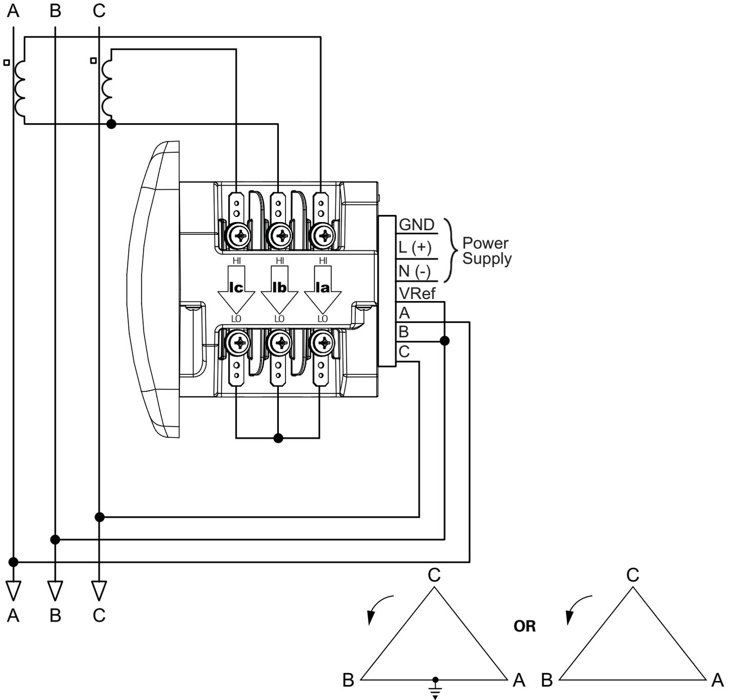
Select: "2 Ct dEL" (2 CT Delta) in Meter Programming setup.
