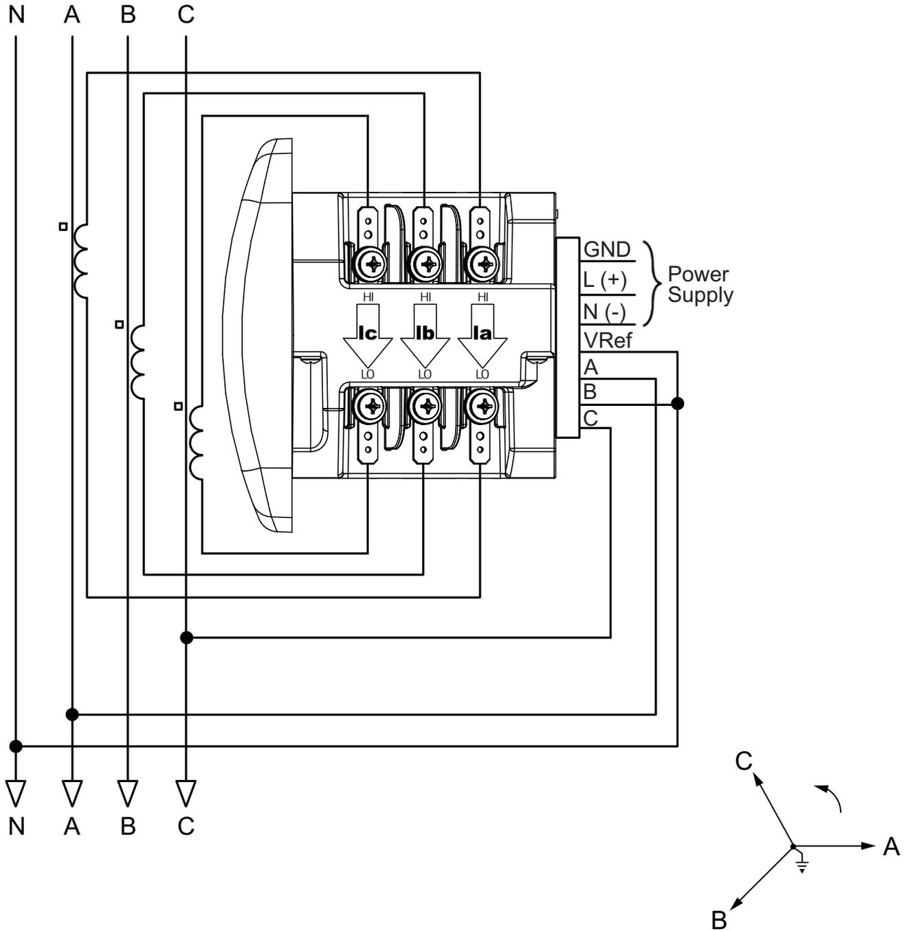
Select: "2.5 EL WYE" (2.5 Element Wye) in Meter Programming setup.
