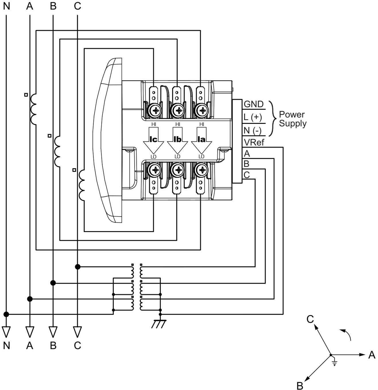
Select: "3 EL WYE" (3 Element Wye) in Meter Programming setup.
