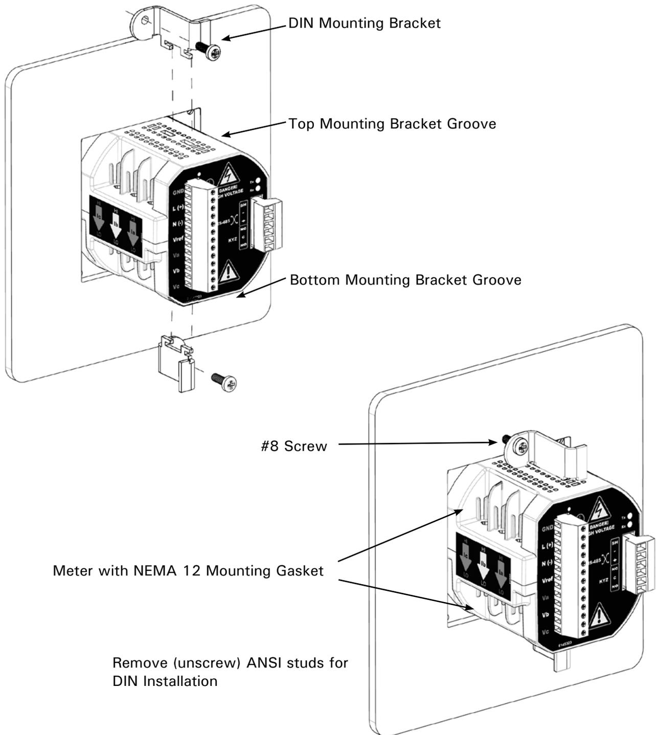
1. Slide the meter with NEMA 12 Mounting Gasket into the panel (first remove ANSI studs, if in place).
