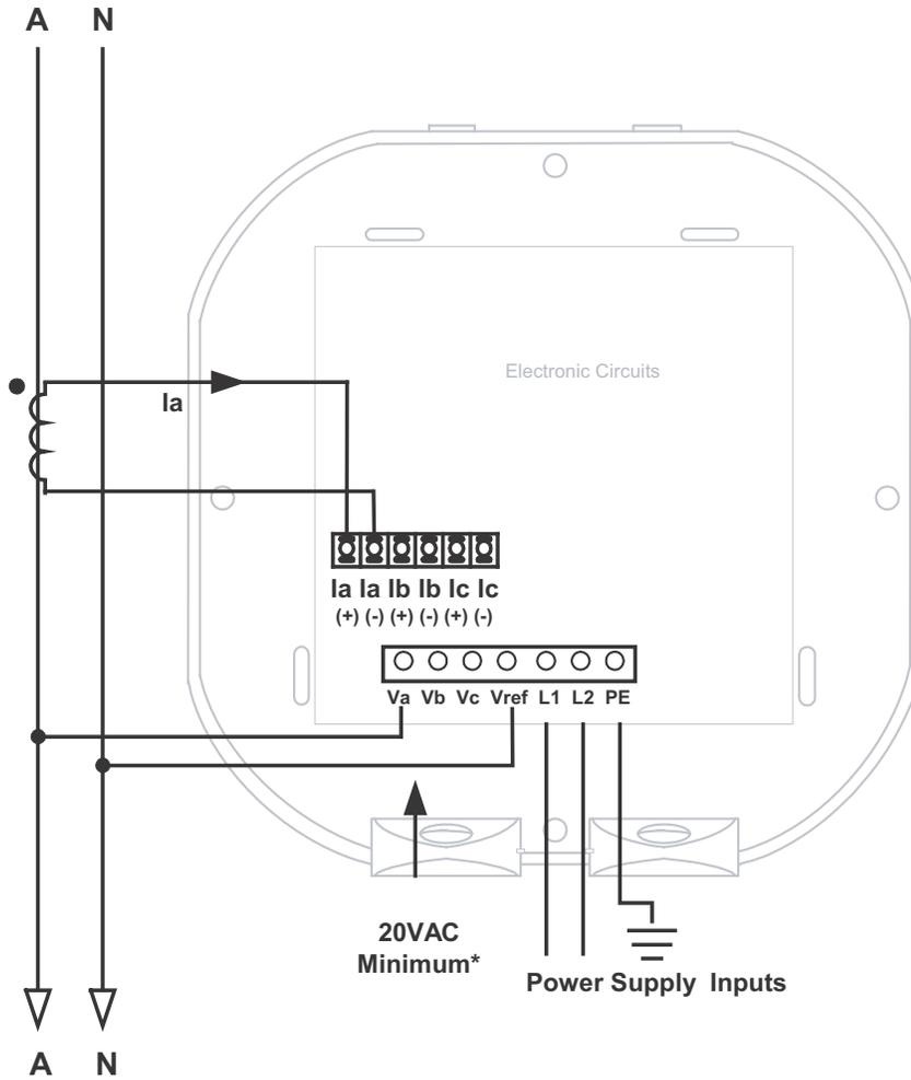
Select: "3 EL WYE" (3 Element Wye) in Meter Programming setup.
