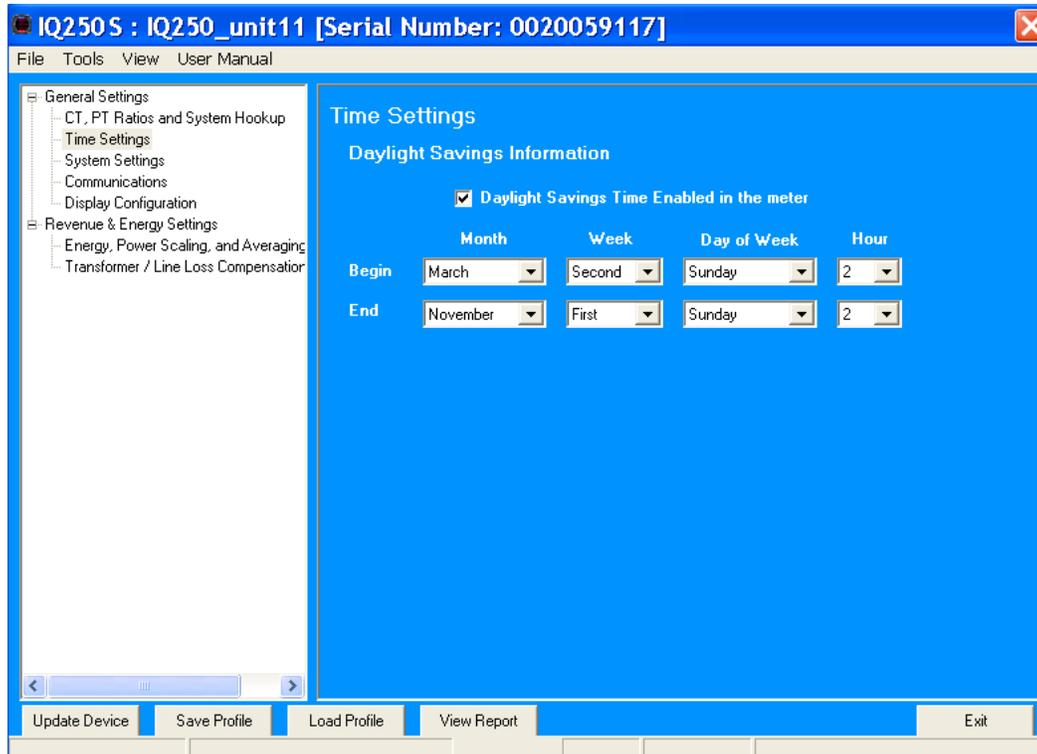
Use this setting to enable or disable Daylight Savings Time for the IQ 250S, and to set the beginning and ending times for Daylight Savings Time. You can also set the Time Zone and enable Clock Sync if supported by your meter.
