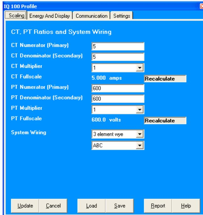
The screenshot shows the 'IQ 100 Profile' window with the 'Scaling' tab selected. The window title is 'IQ 100 Profile' and it has tabs for 'Scaling', 'Energy And Display', 'Communication', and 'Settings'. The main content area is titled 'CT, PT Ratios and System Wiring' and contains the following fields and controls:
