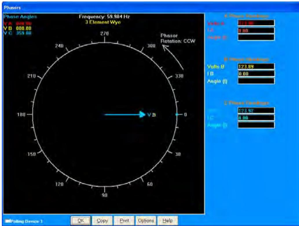
The Phasors screen displays the Phase relationships of the currently connected meter.
