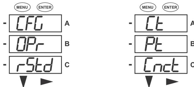
Press **Enter** when CFG is in A window - Parameter screen appears -
