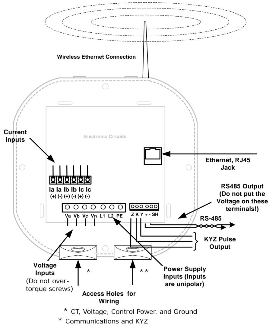
Figure 4.1: Submeter Connections
