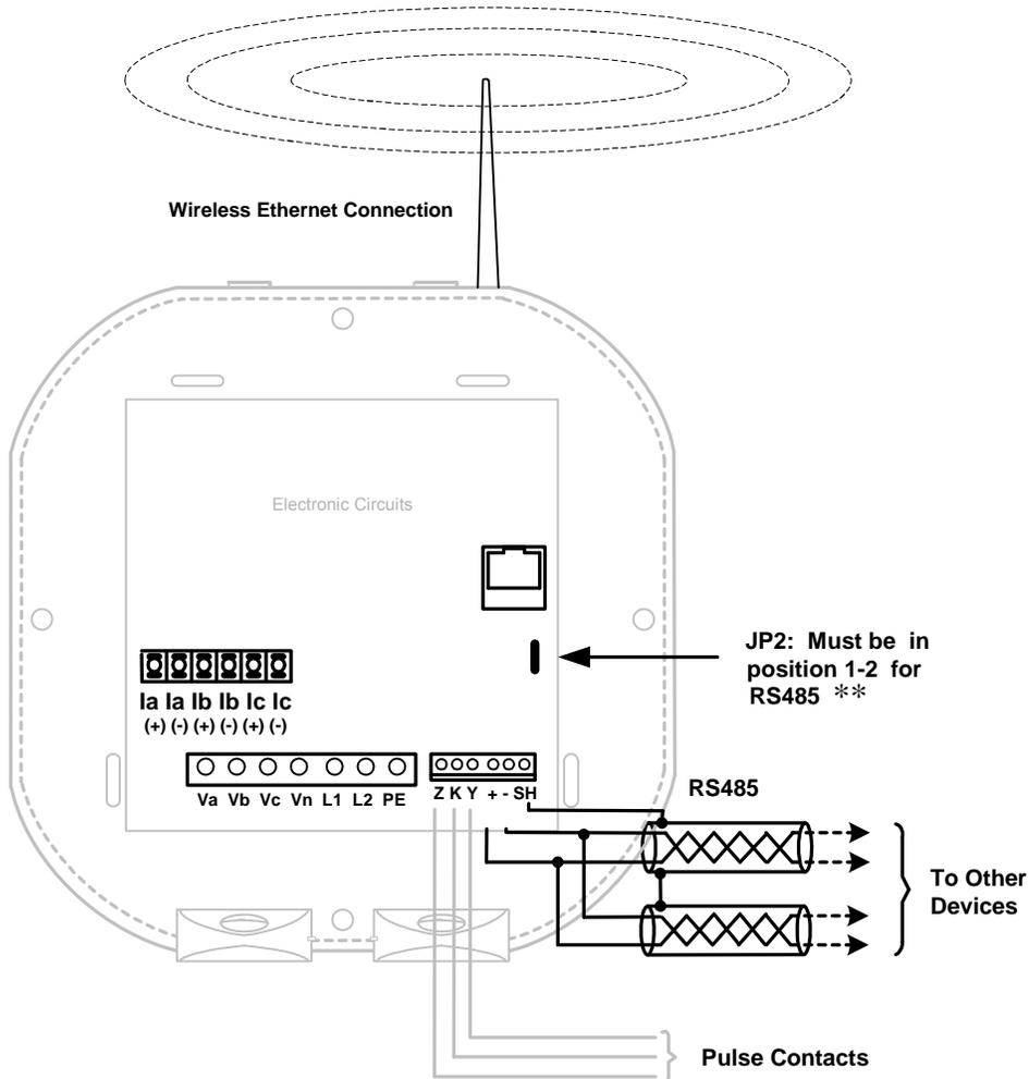
The IQ150S/250S submeter's RS485 connection can be programmed with the buttons on the face of the meter or by using Eaton Meter Configuration software.
