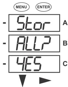
Press the **Enter** button to save the settings. Press the **Right** button for Stor All no screen.
