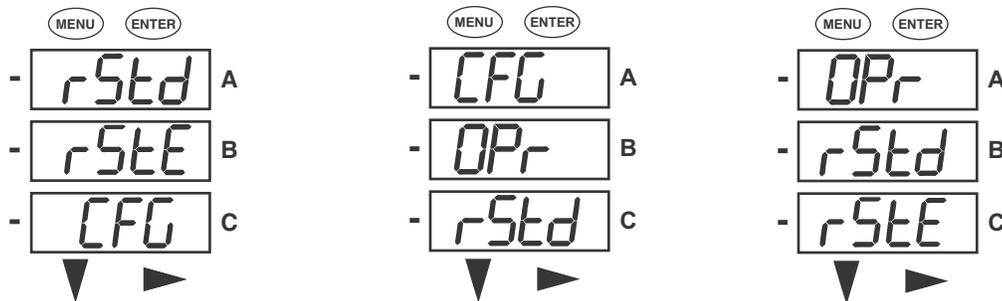
For example: Press Down Twice - CFG moves to A window. Press Down Twice - OPr moves to A window.
