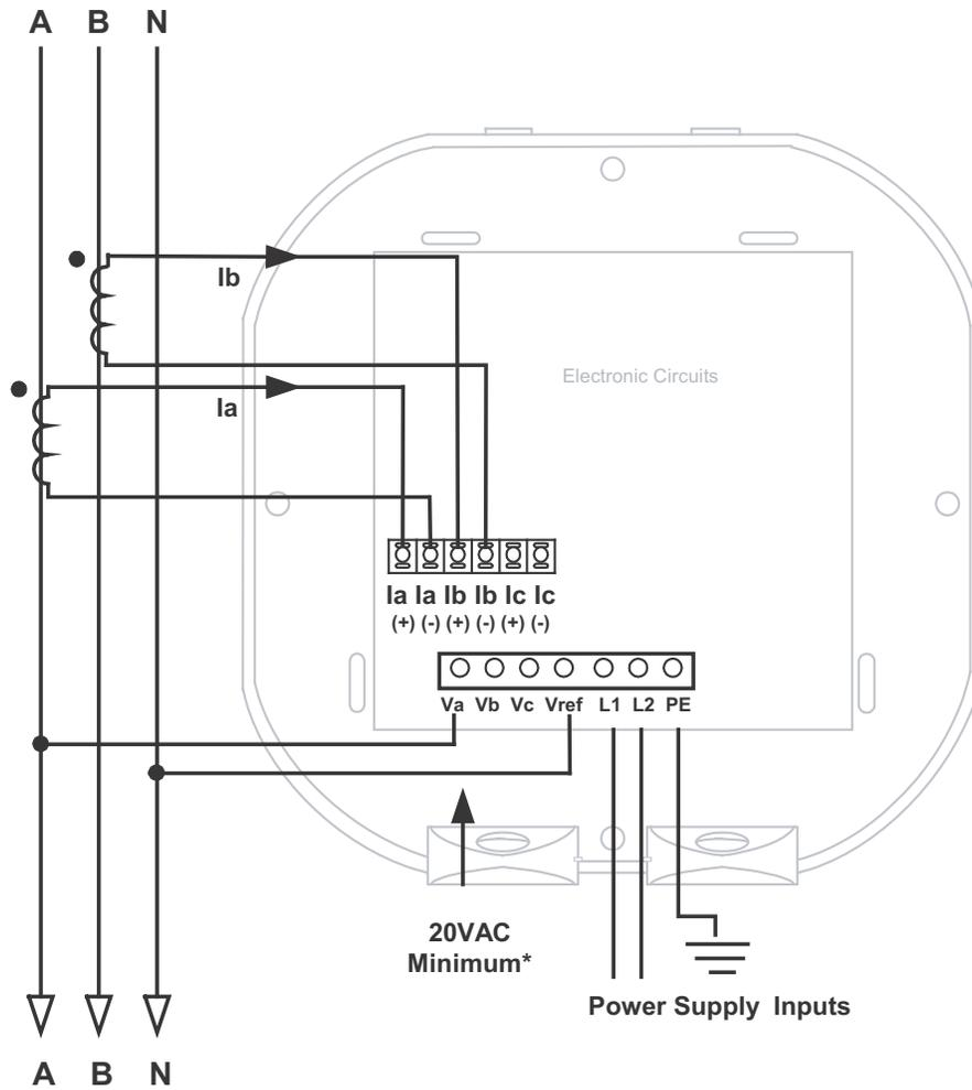
Select: "3 EL WYE" (3 Element Wye) in Meter Programming setup.
