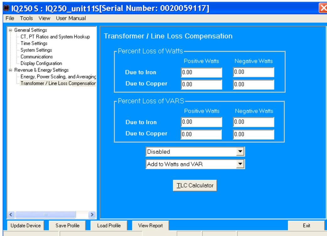
This screen displays the current values for the meter's Transformer Loss Compensation. The screen fields and acceptable entries are as follows
