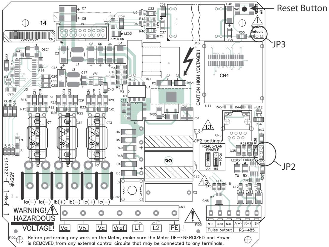
1. Place a shorting block on JP3 and press the **Reset** button on the main board.
