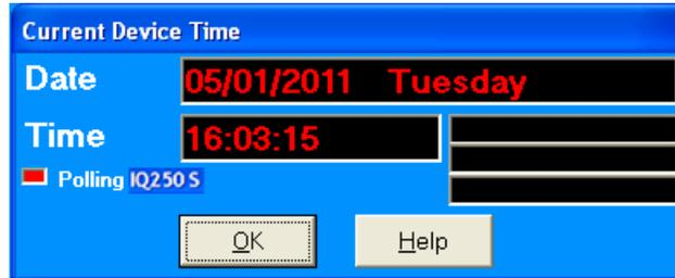
This screen displays the meter's internal time. If Daylight Savings Time is enabled, 'DST' displays in one of the fields to the right of the Time field.
