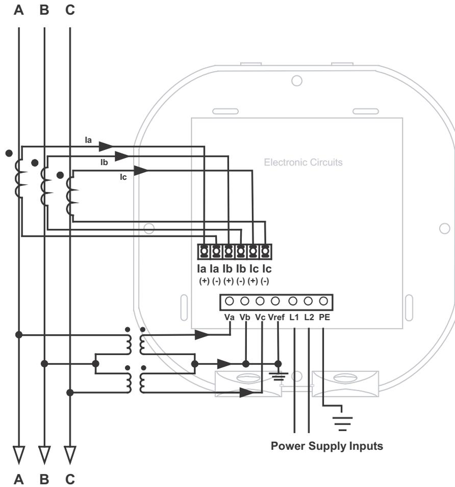
Select: "2 Ct dEL" (2 CT Delta) in Meter Programming setup.
