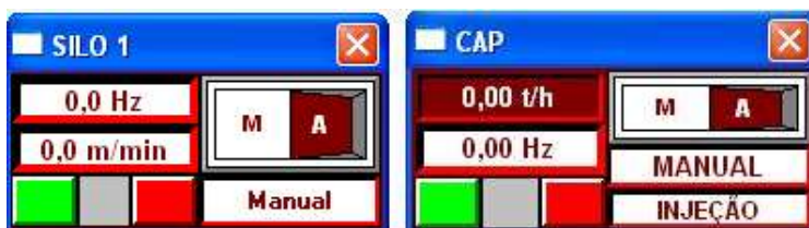
Figure 23 - Example of actuation with frequency inverters
