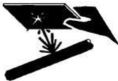
Use a piece of cardboard to detect leaks. Do not use your hands. The fluid injected into the skin must be surgically removed within hours by a doctor familiar with this type of injury, because otherwise, the result may generate a gangrene.
