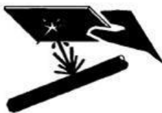
Use a piece of cardboard to detect leaks. Do not use your hands. The fluid injected into the skin must be surgically removed within hours by a doctor familiar with this type of injury, because otherwise, the result may generate a gangrene.
