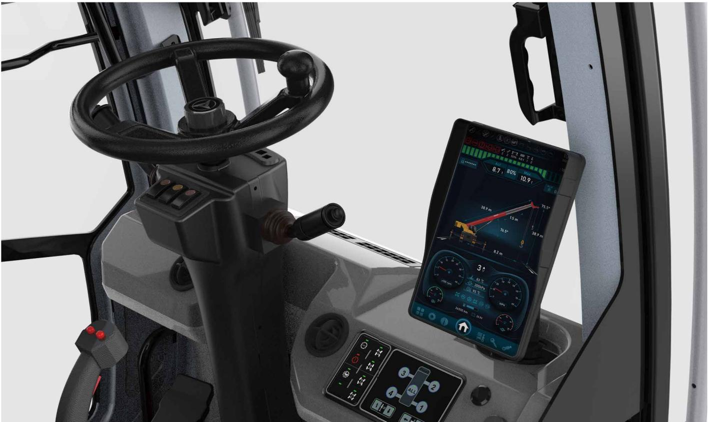
The 10.1" touch screen inserted with optical sensor can automatically adjust the lightness of screen.
