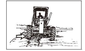
3. Lower the blade horizontally and let it fall to the target cutting depth.
