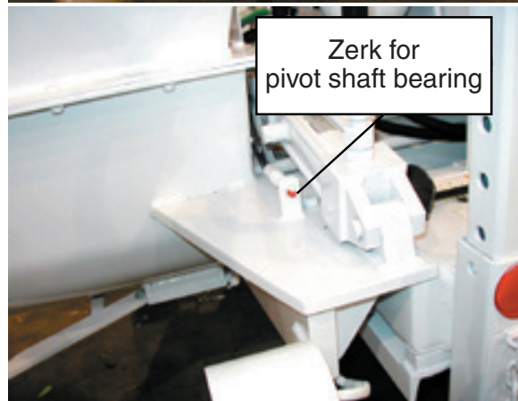
Figure 33 Grease zerks for the outlet assembly and the pivot shaft bearing to be greased each day
