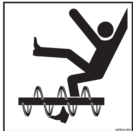
Figure 44 Lifting hopper grate exposes the agitator and the concrete valve
