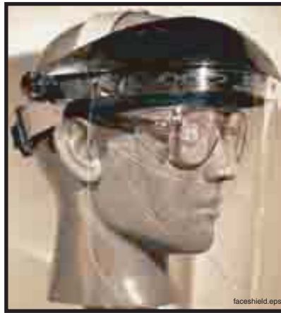
Figure 21 Wear a full face shield for rebound protection
