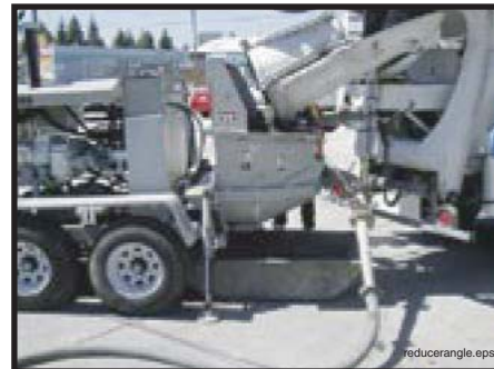
Figure 22 Always point reducers away from the operator and driver
