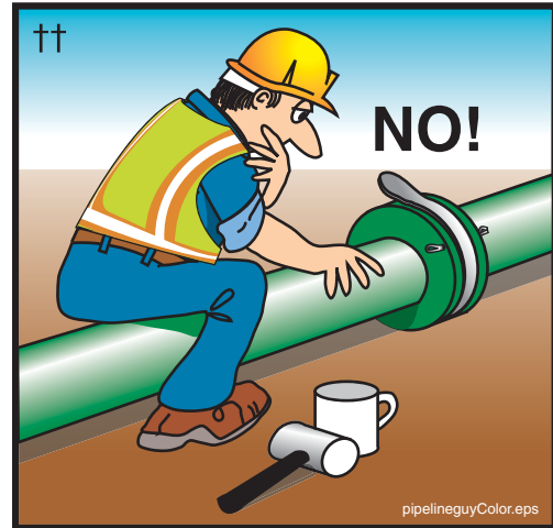
Figure 18 Never straddle or sit on a pressurized pipeline
